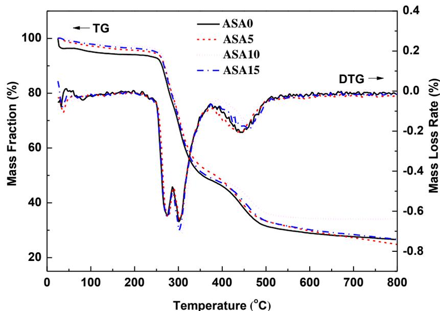
**Fig. 3.** TG/DTG curve of ASA modified eucalyptus/PVC composite
