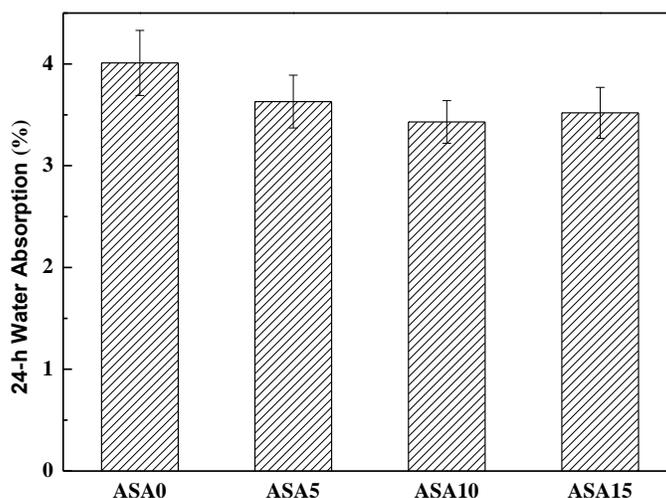
Fig. 4. 24-h Water absorption of ASA modified eucalyptus/PVC composite
