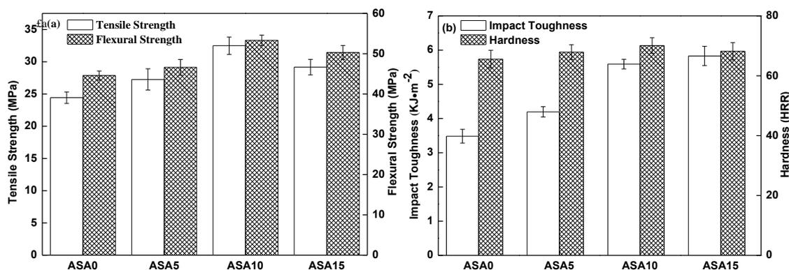
Fig. 1. Mechanical properties of ASA modified eucalyptus/PVC composite
