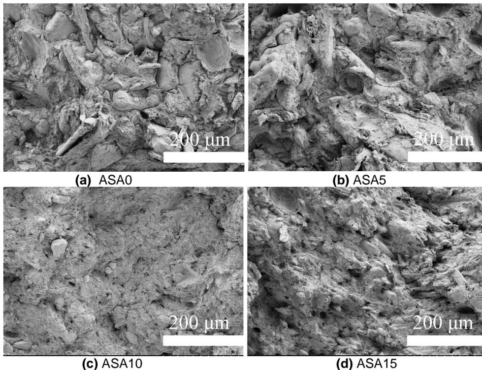
**Fig. 5.** Tensile section micromorphology of ASA modified eucalyptus/PVC composite
