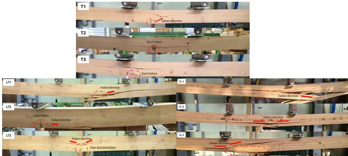
**Fig. 6.** Failure mode of timber, laminated timber, glulam
