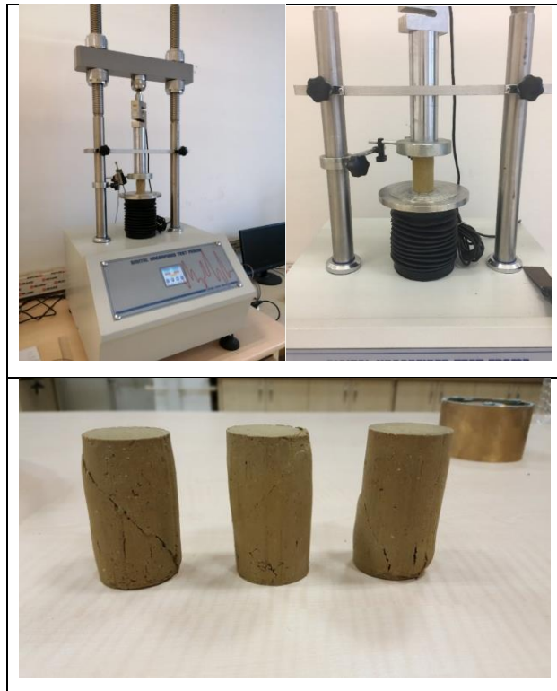
Fig. 3. Unconfined compression test snapshot
