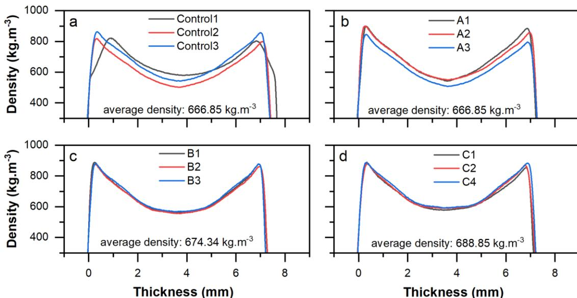
Fig. 5. Density Profiles of DAS-eMDI-MFC bonded MDF Panels. See Table 1 for Panel Codes
