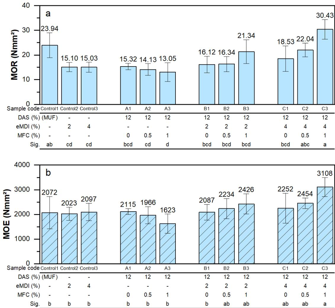
**Fig. 6.** MOR (a) and MOE (b) of the MDF Panels bonded with DAS-based Adhesive Systems in Comparison to Control Panels with MUF or eMDI Adhesives. Ratios (wt%) of DAS, eMDI and MFC are given in the table below the figures. Values in the same column followed by different superscript letters were significantly different ( $p \leq 0.05$ ).
