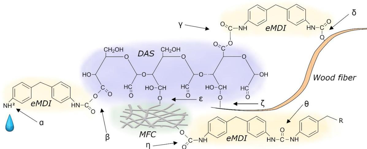
**Fig. 8.** Proposed Bonding Mechanisms of DAS-eMDI-MFC and Wood Fibers in MDF Panels ( $\alpha$ : eMDI-water bonding,  $\beta$ : eMDI-DAS bonding at aldehyde group,  $\gamma$ : eMDI-DAS bonding at OH-group,  $\delta$ : eMDI- wood fiber bonding,  $\epsilon$ : DAS-MFC bonding,  $\zeta$ : DAS-wood fiber bonding,  $\eta$ : eMDI-MFC bonding,  $\theta$ : eMDI-eMDI bonding)
