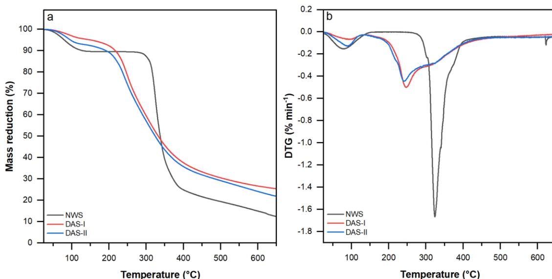
**Fig. 3.** TGA (a) and DTG (b) Curves of Native Wheat Starch (NWS) and Dialdehyde Starch (DAS) Samples
