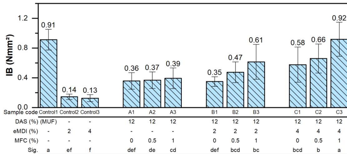
**Fig. 7.** Internal Bond (IB) Strength of MDF Panels bonded with DAS-based Adhesive Systems in Comparison to Control Panels with MUF or eMDI Adhesives. Ratios (wt%) of DAS, eMDI and MFC are given in the table below the figures. Values in the same column followed by different superscript letters were significantly different ( $p \leq 0.05$ ).
