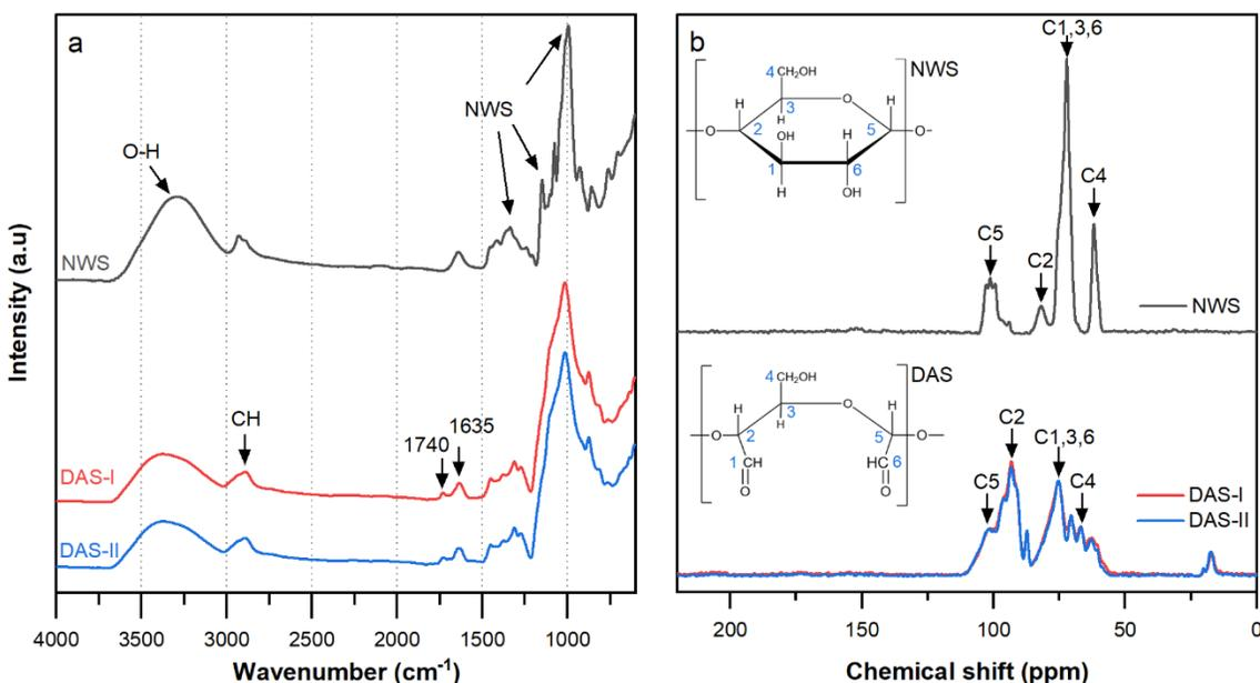
**Fig. 2.** FTIR (a) and  $^{13}\text{C}$ -NMR (b) of Native Wheat Starch (NWS) and Dialdehyde Starch (DAS)
