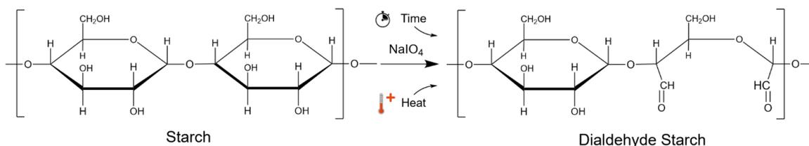
**Fig. 1.** The reaction equation of oxidation of starch with  $\text{NaIO}_4$
