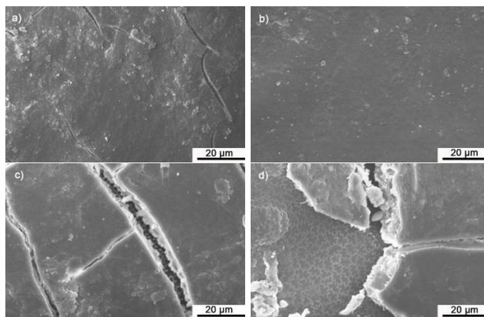
**Fig. 7.** Surface microstructure images of the a) untreated, b) dry heat treated, c) polished, and d) combined treated SC
