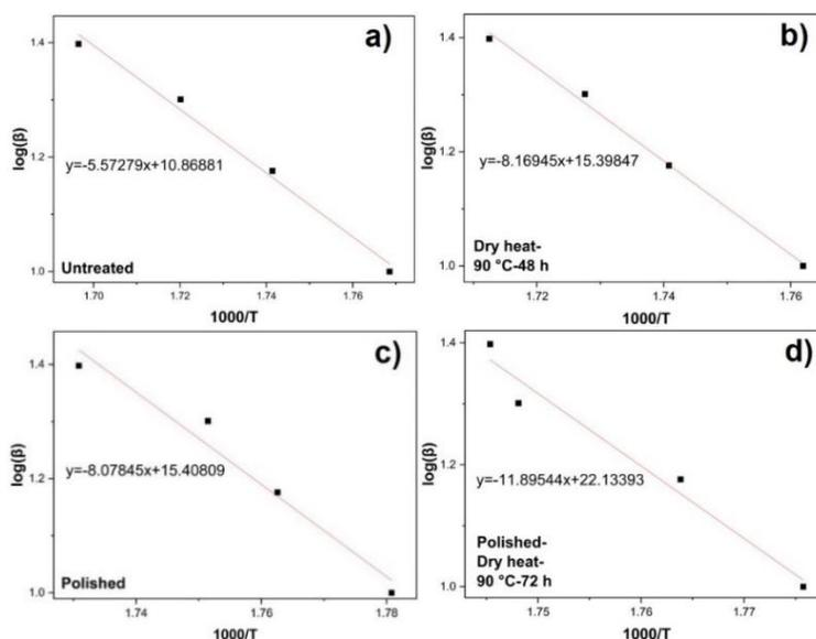
**Fig. 6.** Linear fitting of  $\log(\beta)$  with  $1/T$  for the SC that were a) untreated, b) dry heat treated at 90 °C for 48 h, c) polished, and d) polished and dry heat treated at 90 °C for 72 h
