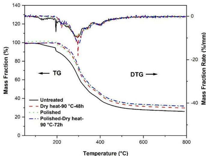
**Fig. 5.** The TG/DTG curves of four kinds of the preprocessed SC
