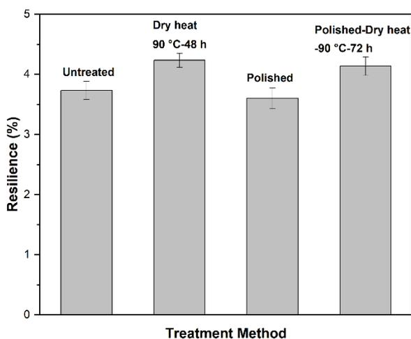
Fig. 8. The resilience of the SC as a filler material
