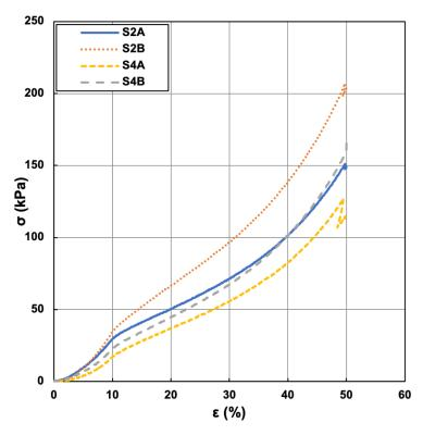
Fig. 3. Stress  $(\sigma)$  – strain  $(\varepsilon)$  curve until 50% strain for samples S2A, S2B, S4A, and S4B
