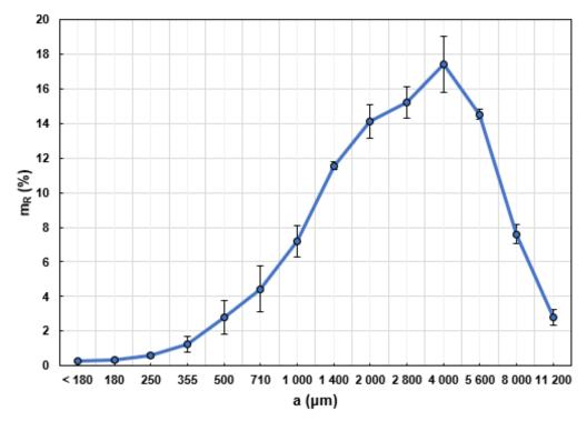
**Fig. 2.** The mass fraction of retained CSs  $(m_R)$  with residuals, *i.e.*, mass losses considered per sieve size (a); error bars depict the sample standard deviations of the retained mass fractions
