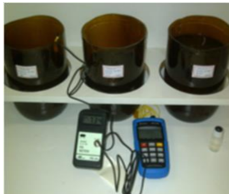
Fig. 1. Fabricated prototype for the biological soaking process
