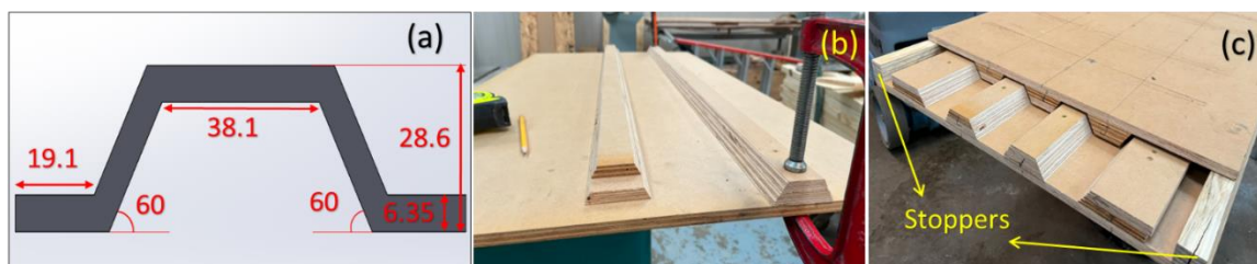
Fig. 2. (a) Dimensions of the corrugated geometry in mm, (b) mold's parts during assembly, and (c) final wooden mold with stoppers on both sides
