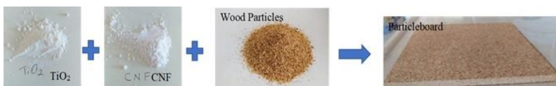
Fig. 1. Raw materials used in particleboard production
