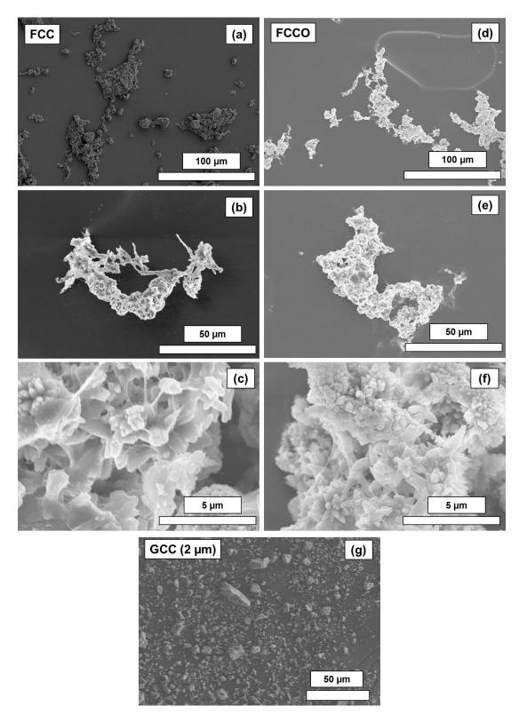
**Fig. 2.** Micrographs of flexible calcium carbonate from MFC (FCC, a toc), and MFCO (FCCO, d to f). and GCC (g). The images (b), (e) and (c), (f) are high magnification of 1K, and 10K, respectively for each FCC.
