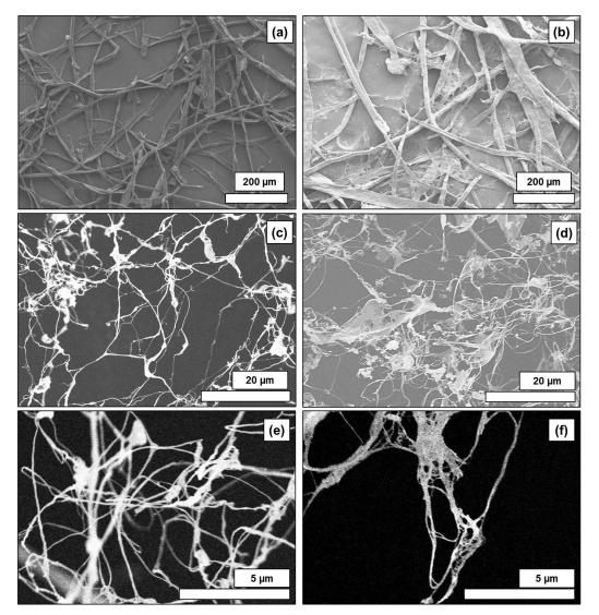
**Fig. 1.** SEM images of the HwBKP (a) and OCC (b) and their fibrillated samples; MFC (c) from HwBKP and MFCO (d) from OCC, respectively. Their higher magnifications were also shown in MFC (e) and MFCO (f).
