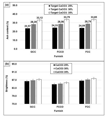
Fig. 3. Ash content (a) and brightness (b) of the papers containing three different fillers
