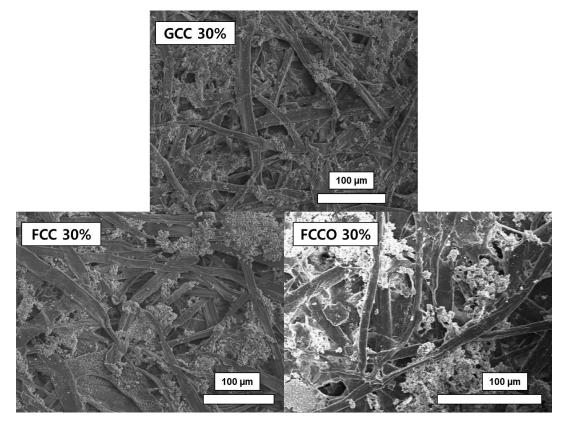
Fig. 4. Typical SEM images of GCC, FCC, FCCO-containing paper with the ash content of 30%
