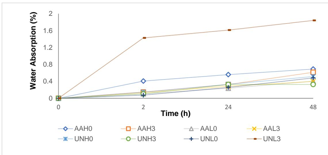
**Fig. 3.** The effect of fiber treatment with acetic anhydride and MAPP content on water absorption
