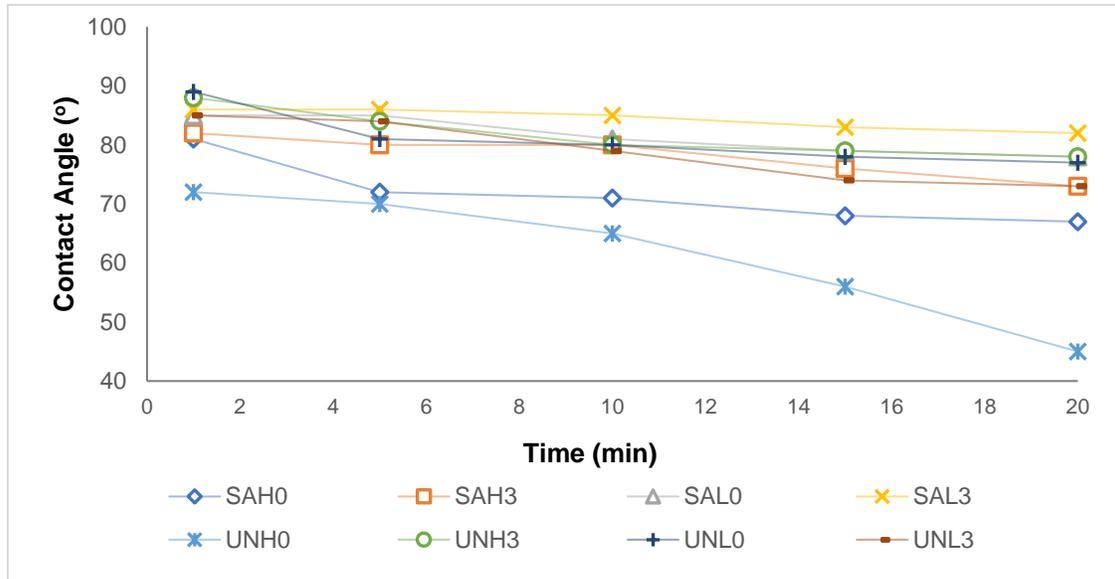
**Fig. 8.** The effect of fiber treatment with acetic anhydride and MAPP content on water contact angle
