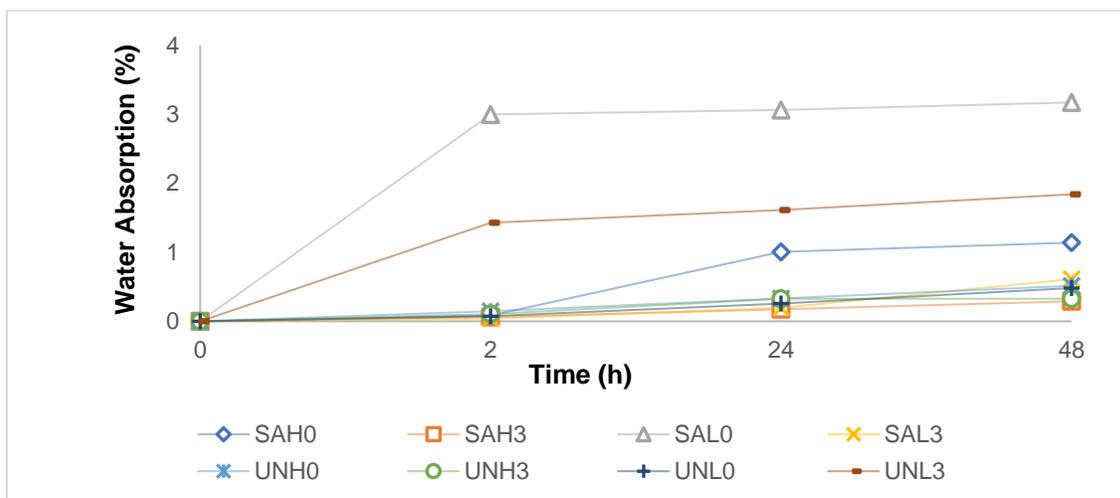
**Fig. 4.** The effect of fiber treatment with succinic anhydride and MAPP content on water absorption
