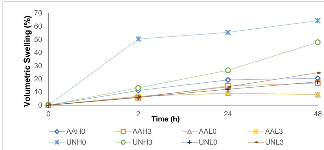
**Fig. 5.** The effect of fiber treatment with acetic anhydride and MAPP content on volumetric swelling
