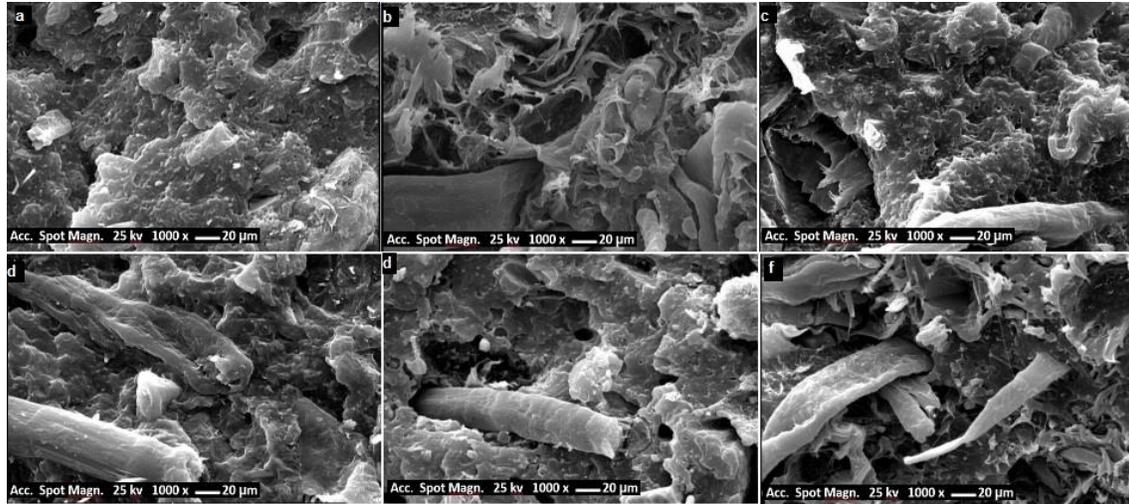
**Fig. 9.** Scanning electron micrographs of the composites filled with modified paper sludge: (a) AAH0, (b) AAL0, (c) SAH0, (d) SAL0, (e) UNH3, and (f) UNL3
