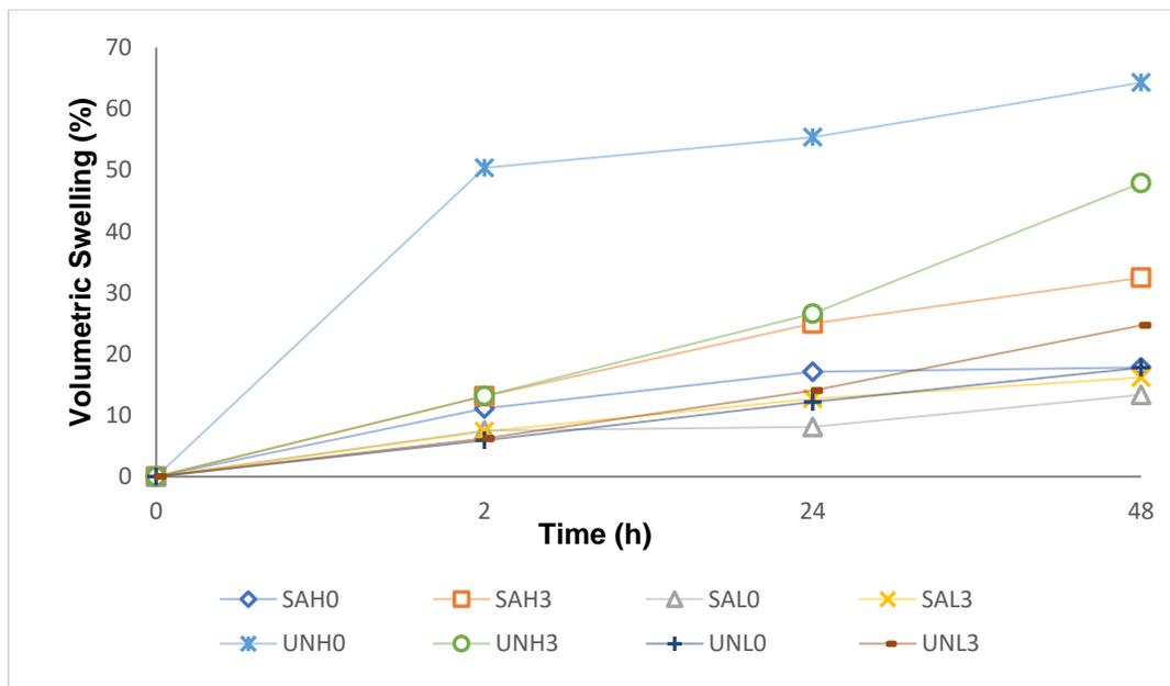
**Fig. 6.** The effect of fiber treatment with succinic anhydride and MAPP content on volumetric swelling
