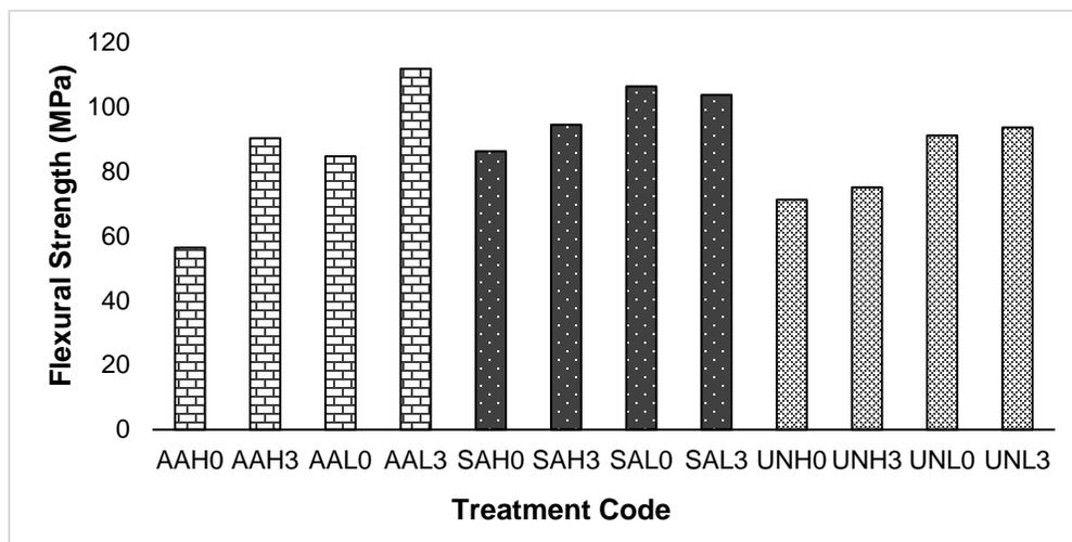
**Fig. 11.** The effect of fiber treatment with succinic anhydride and acetic anhydride polypropylene and MAPP content on flexural strength values of biocomposite
