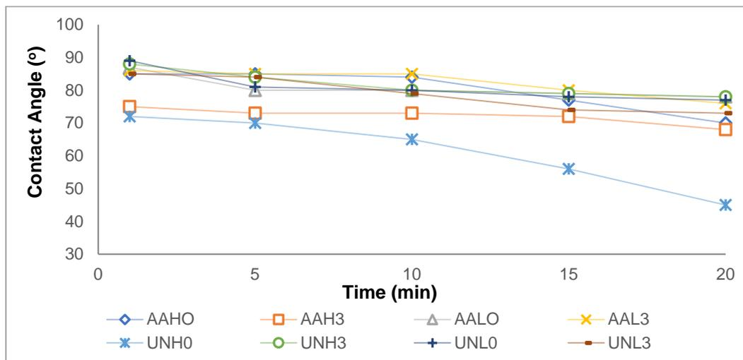
**Fig. 7.** The effect of fiber treatment with acetic anhydride and MAPP content on water contact angle
