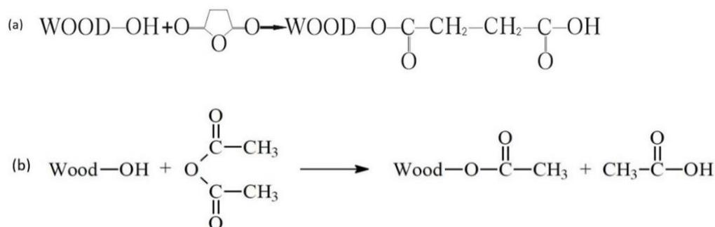
Fig. 1. The reaction of wood with (a) succinic anhydride and (b) acetic anhydride
