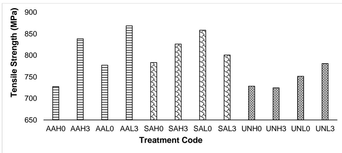
**Fig. 10.** The effect of fiber treatment with acetic anhydride and succinic anhydride, polypropylene and MAPP content on Tensile strength values of biocomposite
