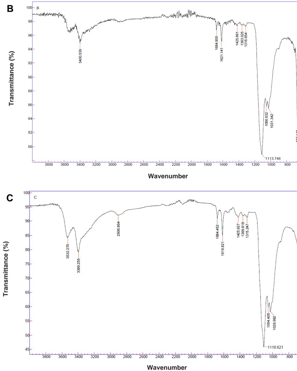
**Fig. 2.** FTIR spectra of untreated (a), acetic anhydride-modified (b), and succinic anhydride-modified (c) paper sludge
