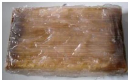
**Fig. 14.** Water penetration by the end face of the sample
