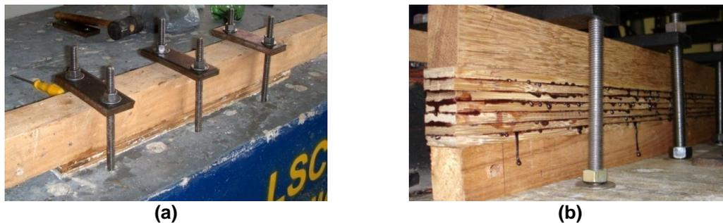
Fig. 2. Pressing process for both glues: a) PVAc; b) PRF
