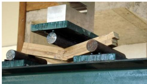
**Fig. 22.** Bending specimen rupture
