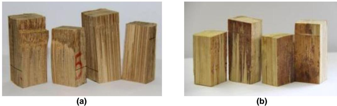
**Fig. 20.** Shear failure mode: (a) Shear parallel to bamboo fiber direction; (b) Shear parallel to GLB glue surface
