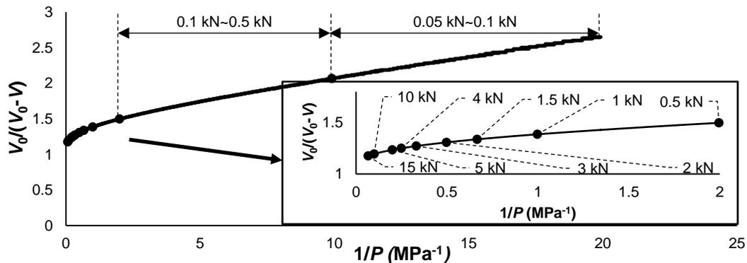
Fig. 3. Curve of the data processed by Kawakita equation
