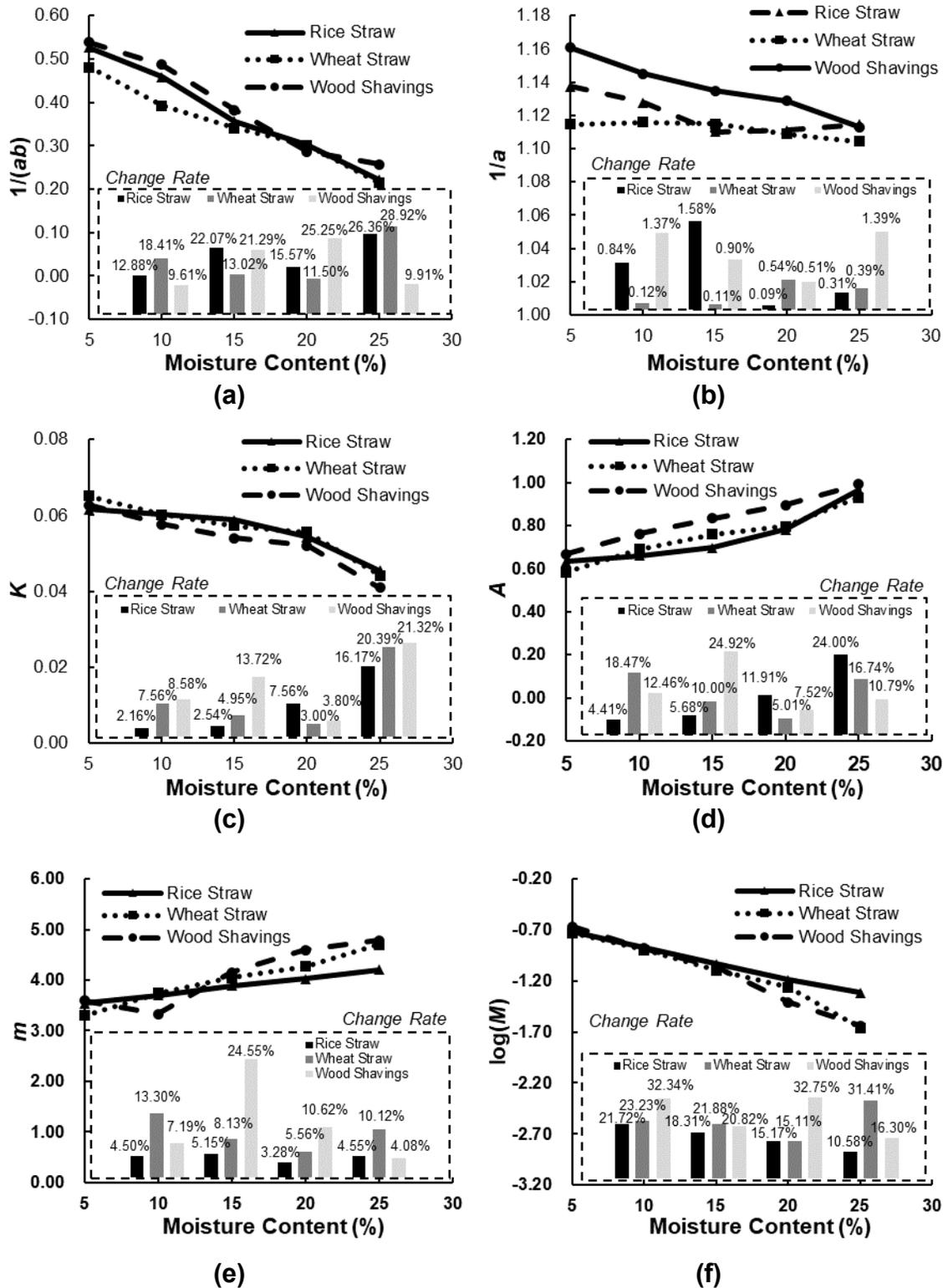
**Fig. 7.** Effects of the moisture content on the coefficients of Kawakita equation, Heckel equation, and Peiyun Huang equation: (a) the coefficient of  $1/(ab)$ ; (b) the coefficient of  $1/a$ ; (c) the coefficient of  $K$ ; (d) the coefficient of  $A$ ; (e) the coefficient of  $m$ ; (f) the coefficient of  $\log(M)$
