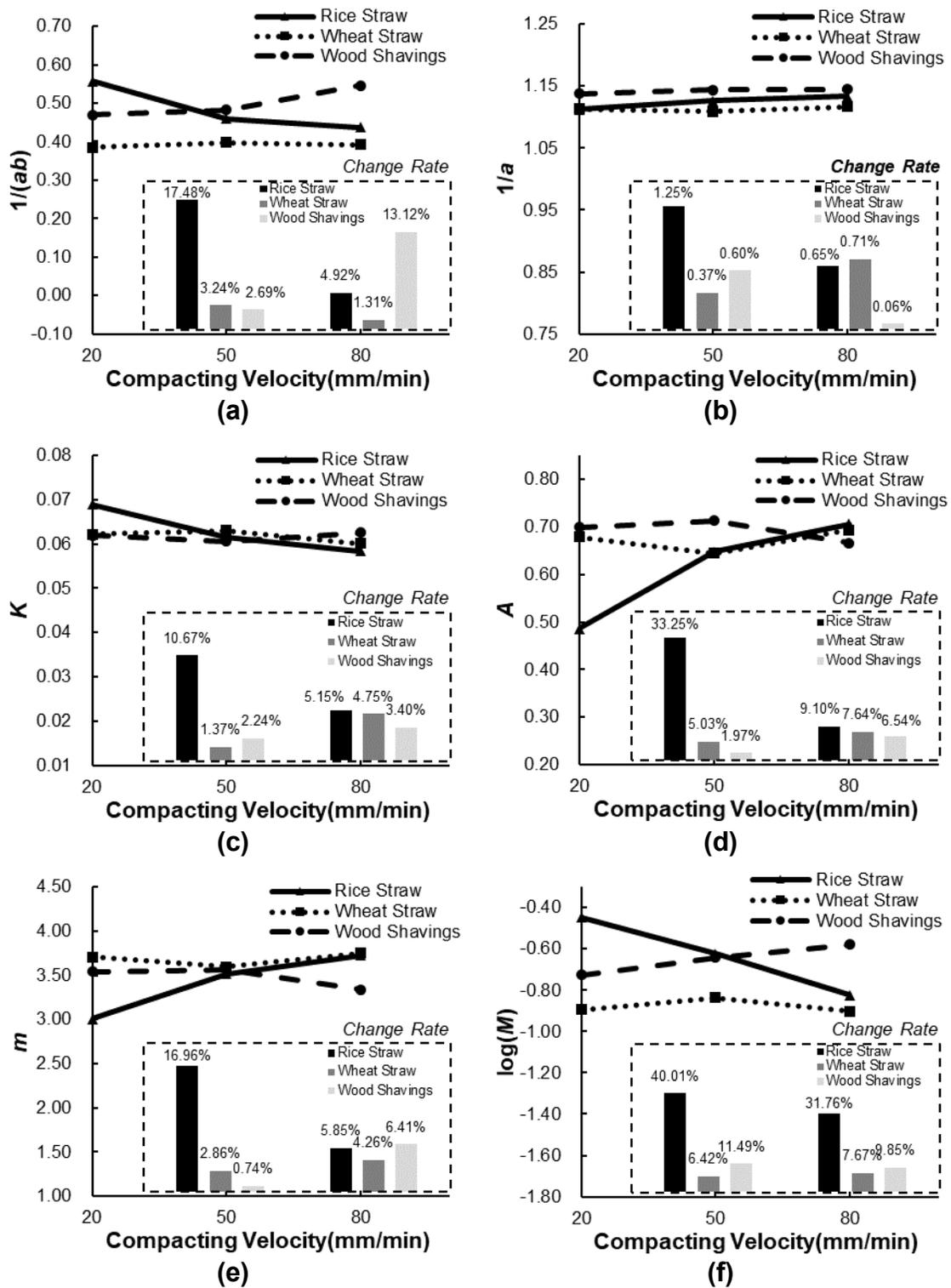
**Fig. 8.** Effects of the compacting velocity on the coefficients of Kawakita equation, Heckel equation, and Peiyun Huang equation: (a) the coefficient of  $1/(ab)$ ; (b) the coefficient of  $1/a$ ; (c) the coefficient of  $K$ ; (d) the coefficient of  $A$ ; (e) the coefficient of  $m$ ; (f) the coefficient of  $\log(M)$
