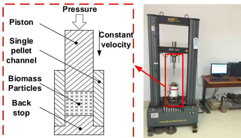
Fig. 1. Test device with a single pellet unit
