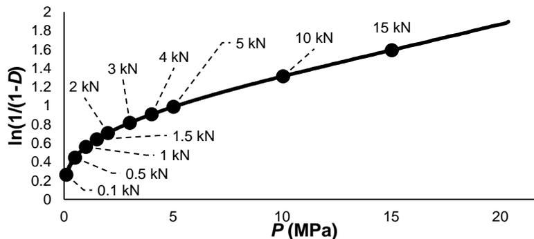
Fig. 4. Curve of the data processed by Heckel equation
