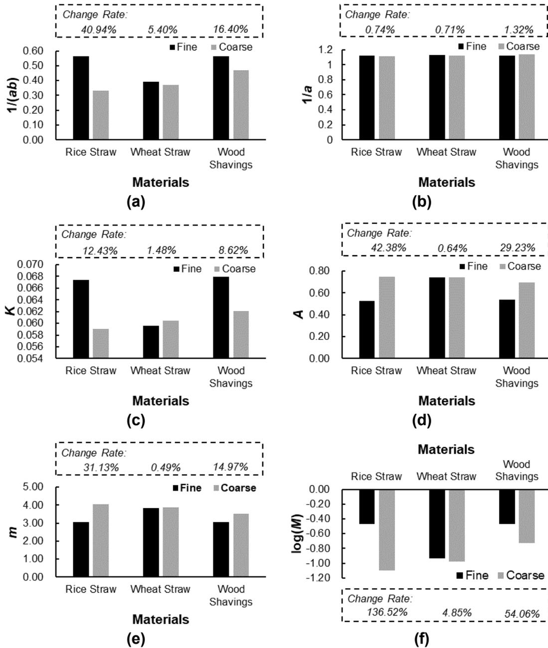
**Fig. 9.** Effects of the particle size on the coefficients of Kawakita equation, Heckel equation, and Peiyun Huang equation: (a) the coefficient of  $1/(ab)$ ; (b) the coefficient of  $1/a$ ; (c) the coefficient of  $K$ ; (d) the coefficient of  $A$ ; (e) the coefficient of  $m$ ; (f) the coefficient of  $\log(M)$
