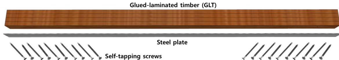
Fig. 1. Separable glued-laminated timber-steel beam
