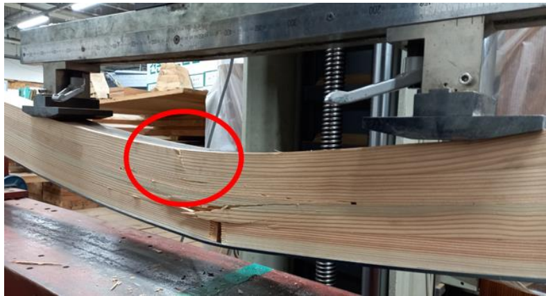
(b) Compression failure on top of GLT
