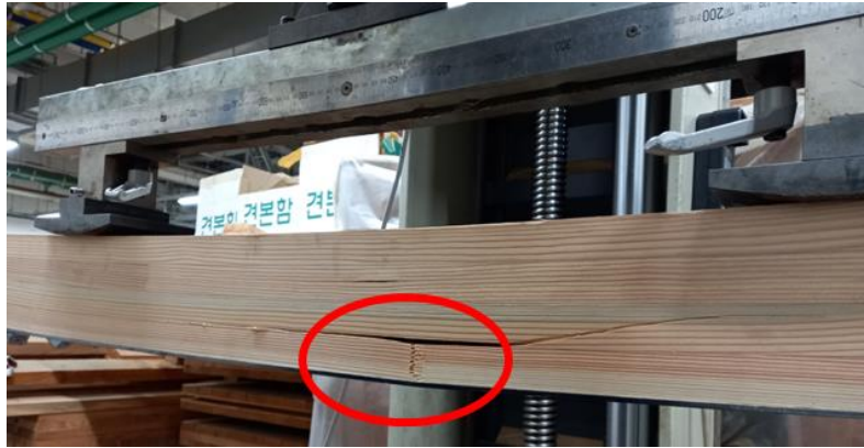
(a) Tensile failure at finger joint of GLT
