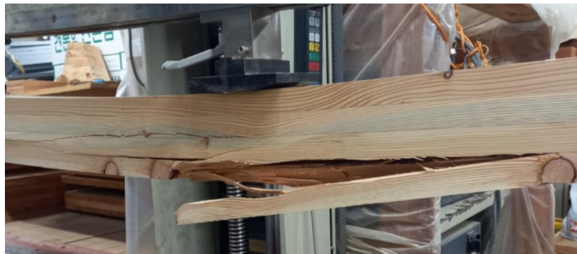
(b) Tensile failure around knot at the bottom lamina
