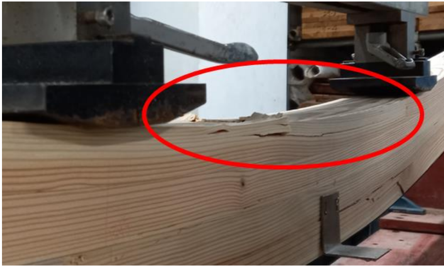
(b) Compression failure on top of GLT
