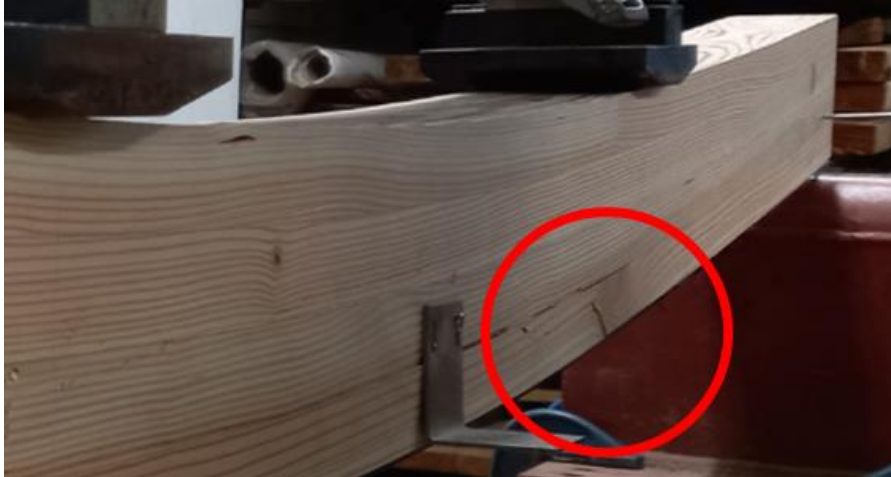
(a) Tensile failure at knot of GLT
