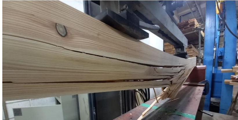
(a) Tensile failure of the bottom lamina
