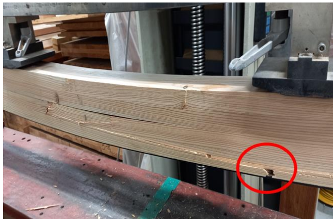
(b) Tension failure on bottom of GLT
