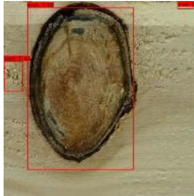
Fig. 8. Illustration of false positives caused by texture distortion or rough surface
