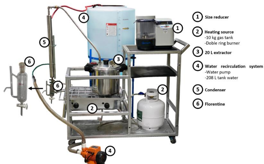
Fig. 1. Essential oil extraction system
