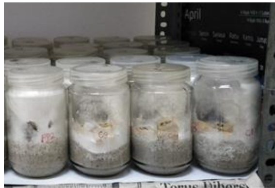
Fig. 3. Test unit of decay attack on the sample
