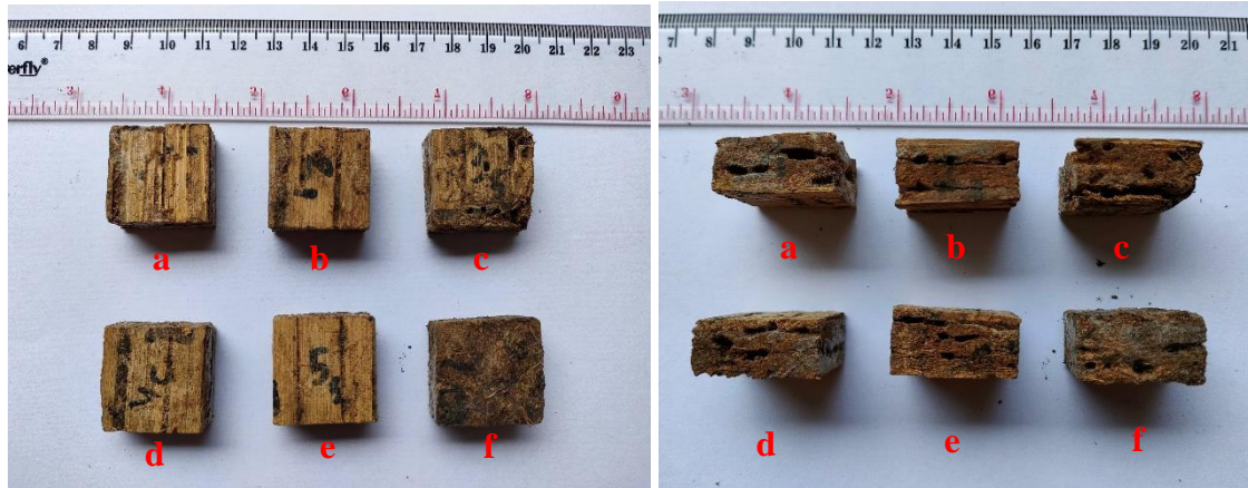
Fig. 6. Visual appearances of particleboard after testing with termites using various bamboo layerings: (a) tali, (b) talang, (c) kuning, (d) belangke, (e) betung, and (f) untreated
