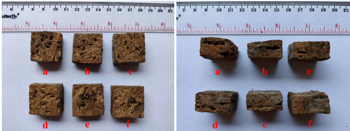
Fig. 4. Visual appearances of particleboard after testing with termites at various compositions of wood shavings: (a) 100/0, (b) 90/10, (c) 80/20, (d) 70/30, (e) 60/40, and (f) 50/50
