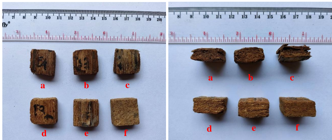
Fig. 7. Visual appearances of particleboard after testing brown-rot decay at various bamboo layerings: (a) tali, (b) talang, (c) kuning, (d) belangke, (e) betung, and (f) untreated
