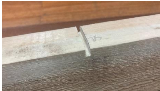
Fig. 1. Rectangular gap of a sample beam
