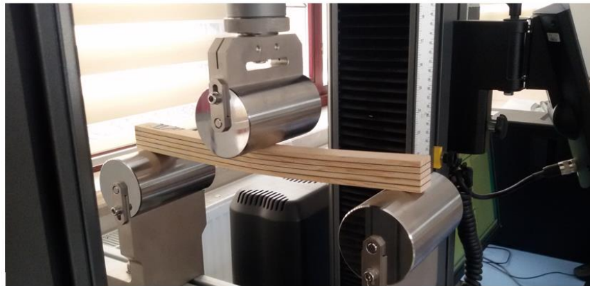
Fig. 4. Scheme of the static bending test
