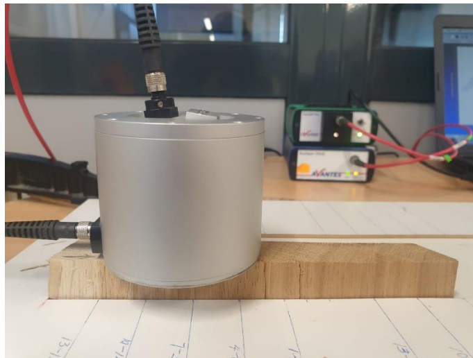
Fig. 3. Color measurement by means of an AvaSpec-USB2 spectrometer (by Avantes Apeldoorn, Netherlands)
