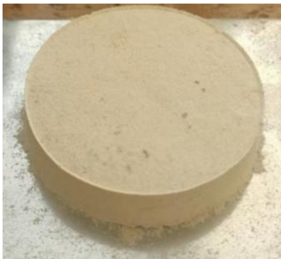
Fig. 4. Preparation of poplar powder specimens
