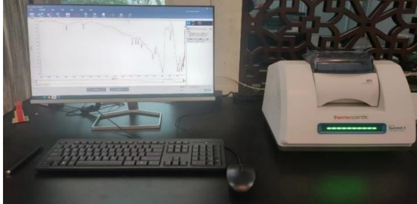
Fig. 7. Physical view of infrared spectroscopic measurements of poplar powder
