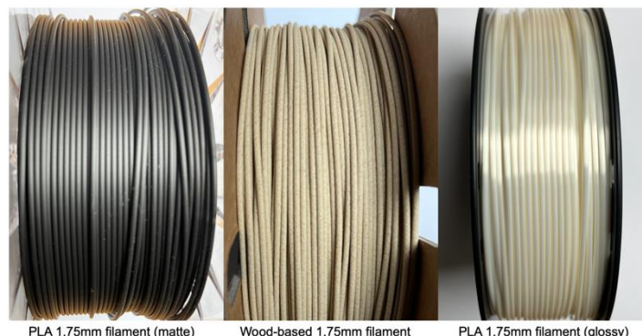
Fig. 1. Example of available wood and PLA-based 1.75 mm filaments
