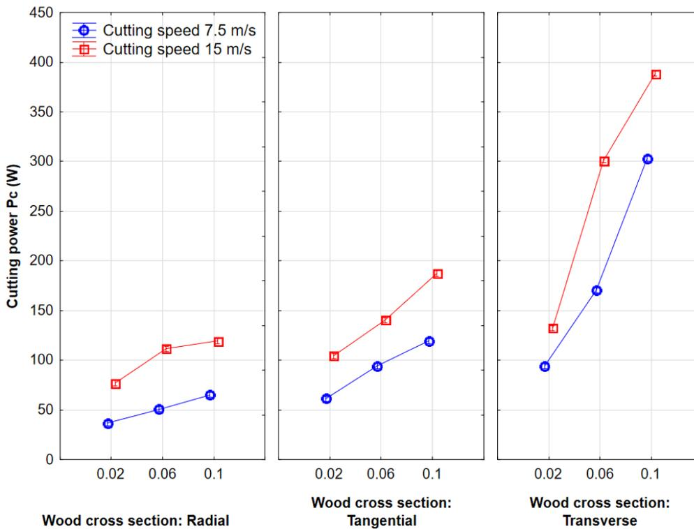
**Fig. 7.** Power cutting as a function of chip thickness, wood cross-section, and cutting speed. Vertical bars denote 95% confidence intervals for the mean.
