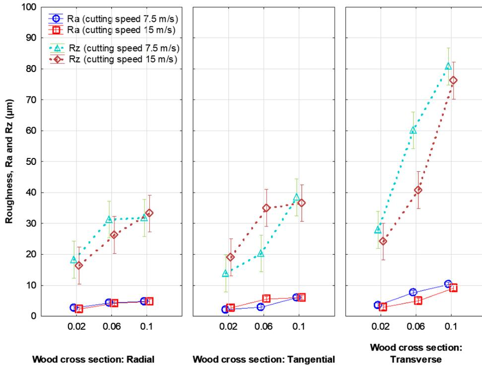
**Fig. 6.** Surface roughness  $R_a$  and  $R_z$  as a function of chip thickness, wood cross-section, and cutting speed. Vertical bars denote 95% confidence intervals for the mean.
