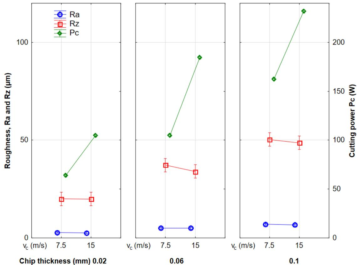
**Fig. 5.** Surface roughness and power cutting as a function of chip thickness and cutting speed. Vertical bars denote 95% confidence intervals for the mean
