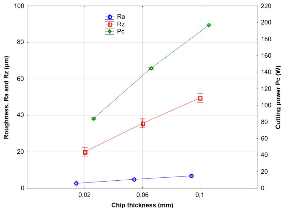
**Fig. 3.** Surface roughness and power cutting as a function of chip thickness. Vertical bars denote 95% confidence intervals for the mean
