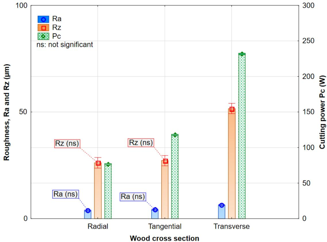
**Fig. 4.** Surface roughness and power cutting as a function of wood cross-section. Vertical bars denote 95% confidence intervals for the mean.
