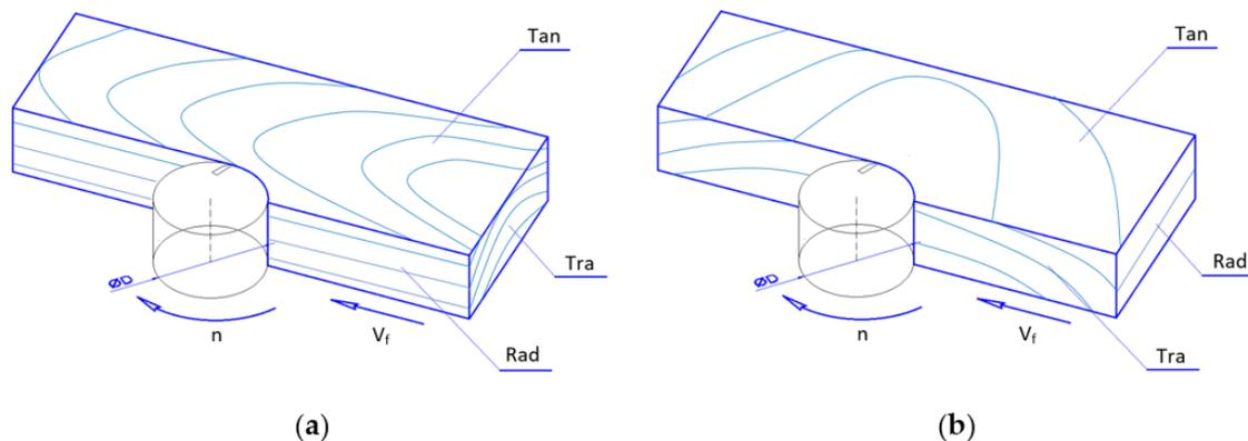
**Fig. 1.** Milling diagram with cross-section variants marked; milling operations at: (a) radial; (b) transverse cross-section;  $v_f$  – feed speed,  $n$  – rotational speed, cross-section: Rad - Radial, Tan - Tangential, Tra - Transverse
