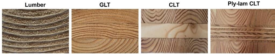
Fig. 1. Representative photographs of tested lumber, GLT, CLT, and Ply-lam CLT
