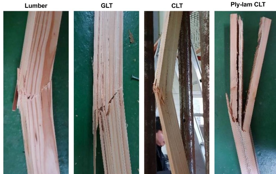
Fig. 9. Failure mode in uninstalled blocking compression test (lumber, GLT, CLT; buckling failure, Ply-lam CLT; buckling+delamination failure)
