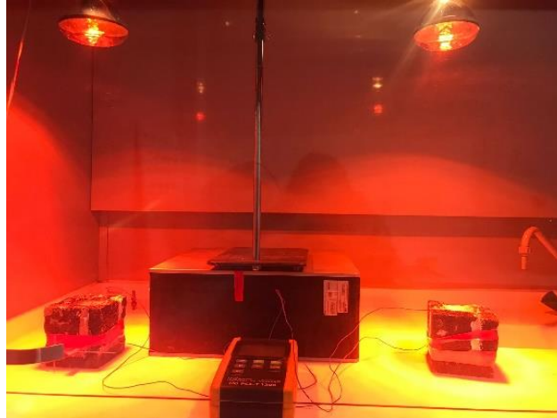
Fig. 1. Lab-scale cubic designs for predicting of thermo-regulative performance of the PCM impregnated wood
