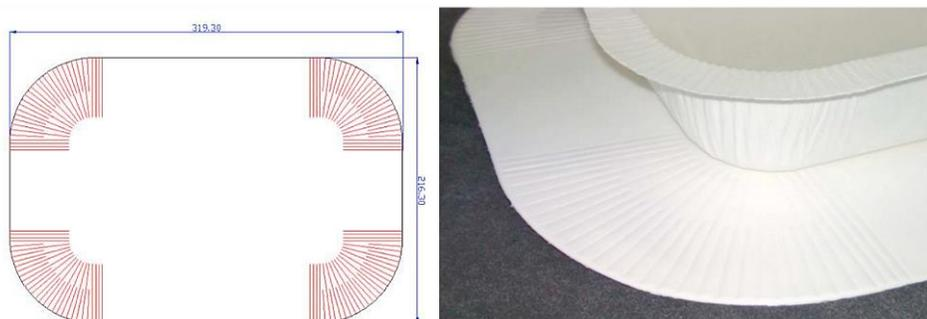
**Fig. 15.** Representation of a tray blank and ready tray. The tray corners are the parts deforming most (Leminen *et al.* 2013).
