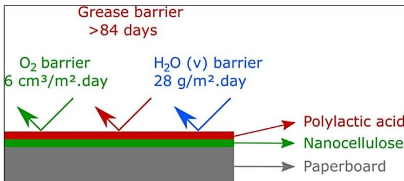
**Fig. 11.** Representation of barrier properties of a novel coated paperboard. Reprinted with permission from Koppolu *et al.* (2019).
