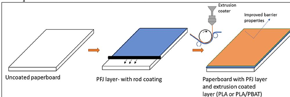
**Fig. 14.** Illustration of multi-layered coating process (Poulose *et al.* 2022). The study is operated under CC-BY license.
