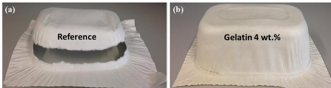
**Fig. 3.** Example of the additive effect on formability: (a) untreated and (b) treated with gelatine paper. Reprinted from Khakalo *et al.*, *Reactive and Functional Polymers* 85, Copyright 2014, with permission from Elsevier.
