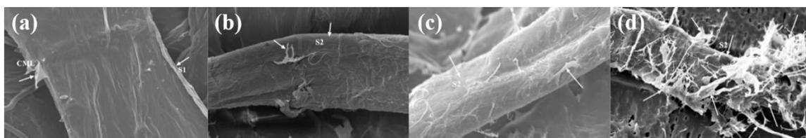
**Fig. 16.** Dependence of fibre surface on beating degree: (a) B0, (b) B2, (c) B4, (d) B7. Modified from Zhao *et al.* (2017), *Carbohydrate Polymers* 174, with permission from Elsevier.
