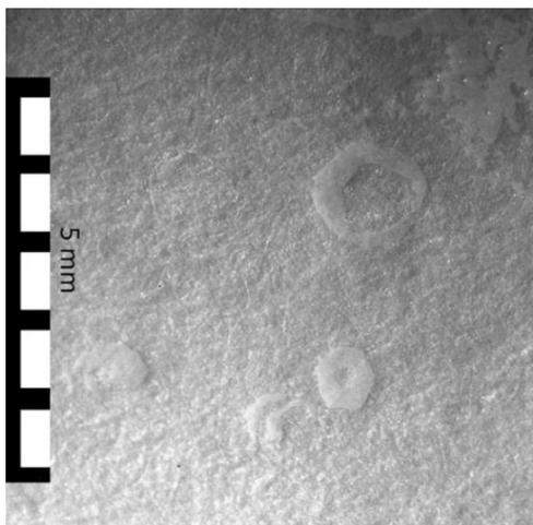
**Fig. 10.** Example of the surface damage due to sticking of the paperboard dispersion coating. Reprinted from Tanninen *et al.* (2014b), with permission from Wiley.
