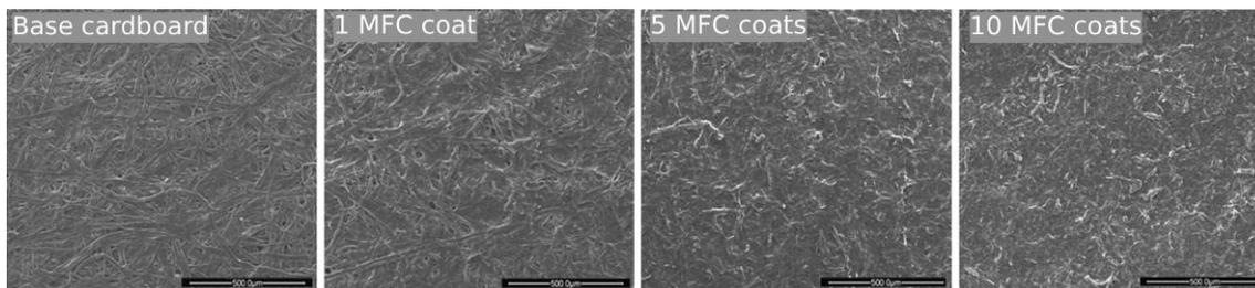
**Fig. 13.** Changes in paperboard surface with increase in the number of coating layers. Modified and reprinted from Lavoine *et al.* (2014), with permission from Wiley.
