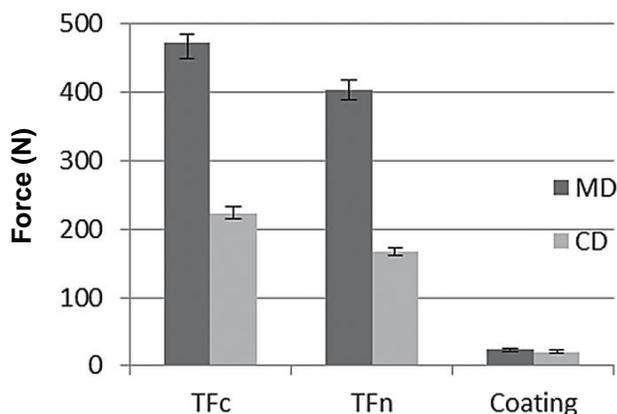
**Fig. 5.** Coating strengthening effect: the force, needed to break a coated sample (TFc) is higher than the sum of the forces needed to break the substrate (TFn) and coating separately. Reprinted from Franke *et al.* (2021) with permission from Wiley.
