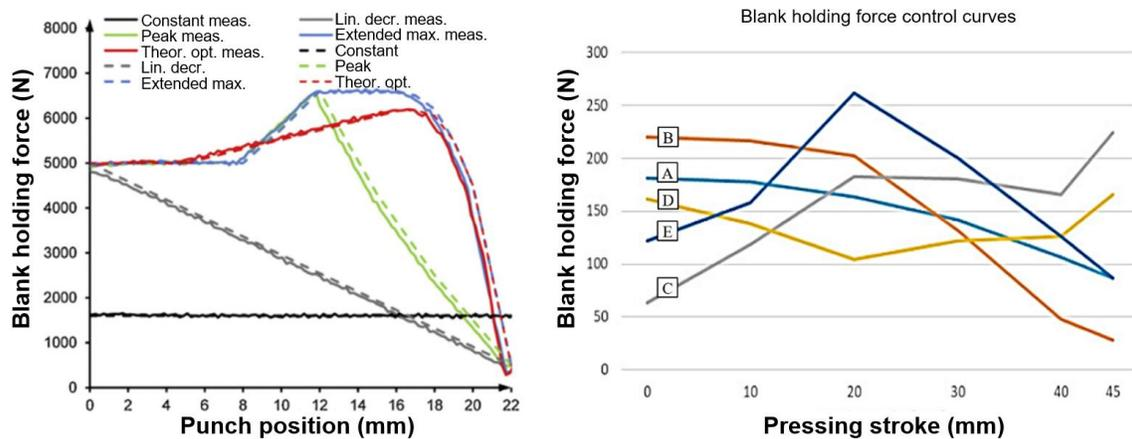
**Fig. 8.** Graphical representation of different BHF trajectories used in tests. Modified from Hauptmann *et al.* (2016), *Journal of Materials Processing Technology* 232 (left), with permission from Elsevier; and Tanninen *et al.* (2020) (right).
