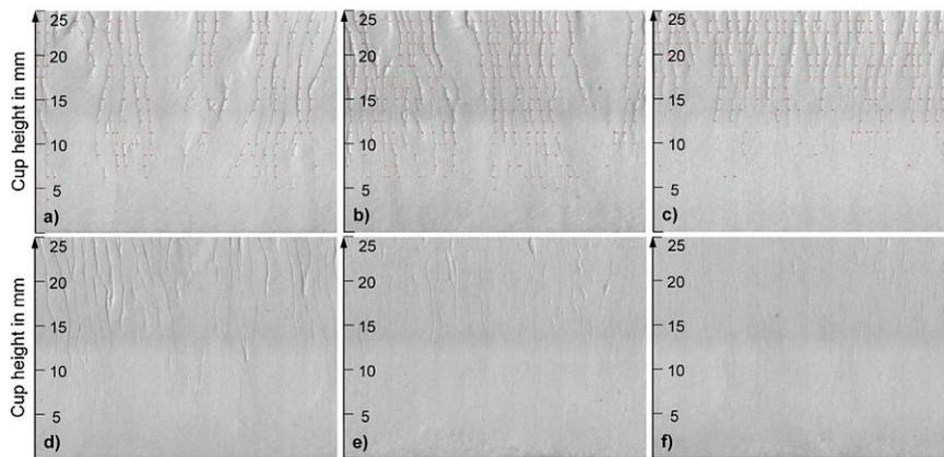
**Fig. 6.** Example of different wall quality after deep drawing using several BHF trajectories. Reprinted from Hauptmann *et al.* (2016), *Journal of Materials Processing Technology* 232, with permission from Elsevier.
