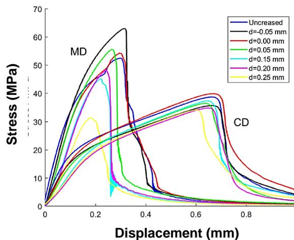
**Fig. 4.** Typical stress-strain graphs for paperboard-based materials: mechanical properties usually differ in the CD and MD directions. Reprinted from Marin *et al.* (2022), with permission from Wiley.
