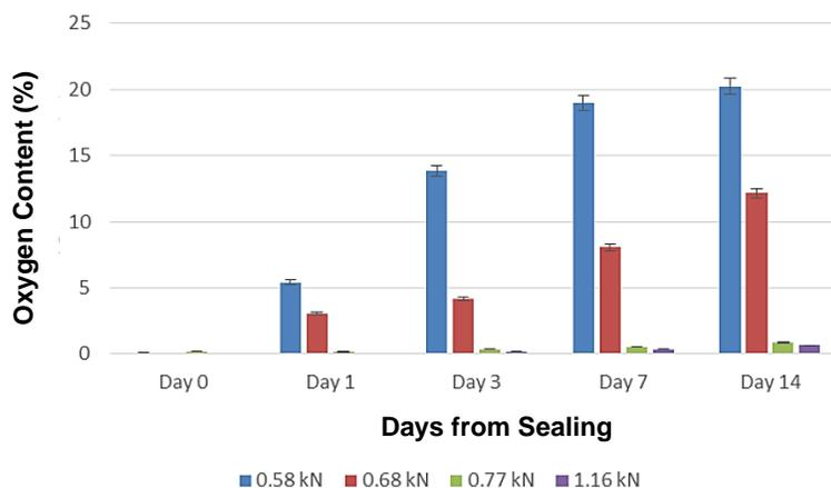
**Fig. 7.** Oxygen content increase inside rectangular trays as an indicator of sealability in response to the BHF value used during forming (Leminen *et al.* 2015).
