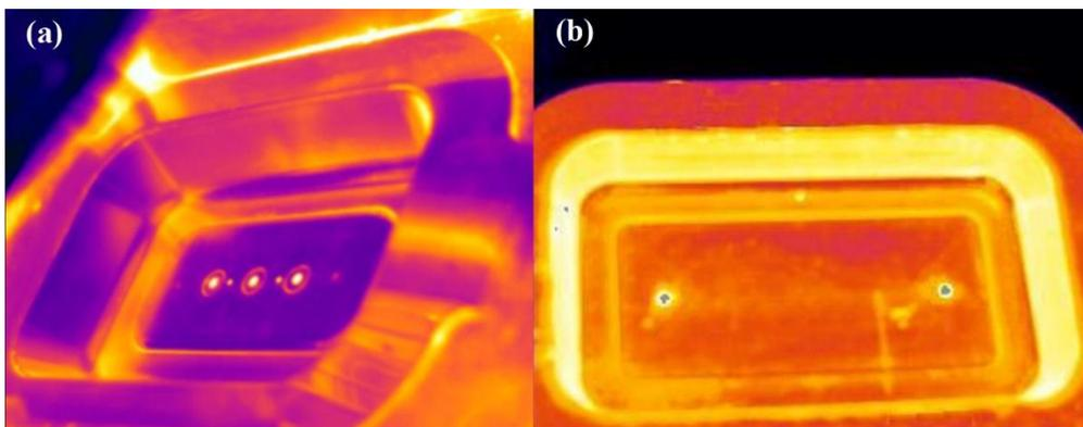
**Fig. 9.** Heat distribution of (a) traditional and (b) improved mould designs. Modified from Tanninen *et al.* (2014a) *Journal of Materials Processing Technology* 214(8), with permission from Elsevier.
