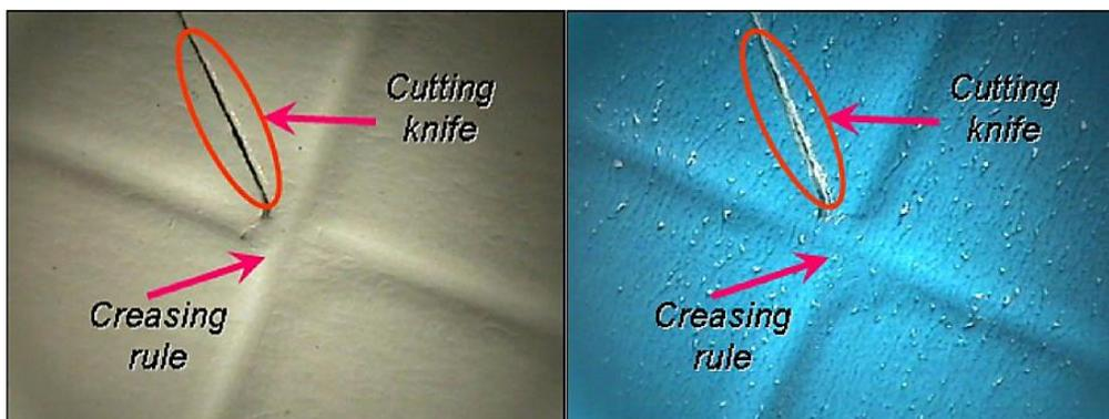
**Fig. 1.** Creasing and cutting lines on the printed and unprinted surface of coated paperboard. Modified from Kim *et al.* (2010); Reprinted from *Journal of Industrial and Engineering Chemistry*, 16(5), Copyright 2010, with permission from Elsevier.
