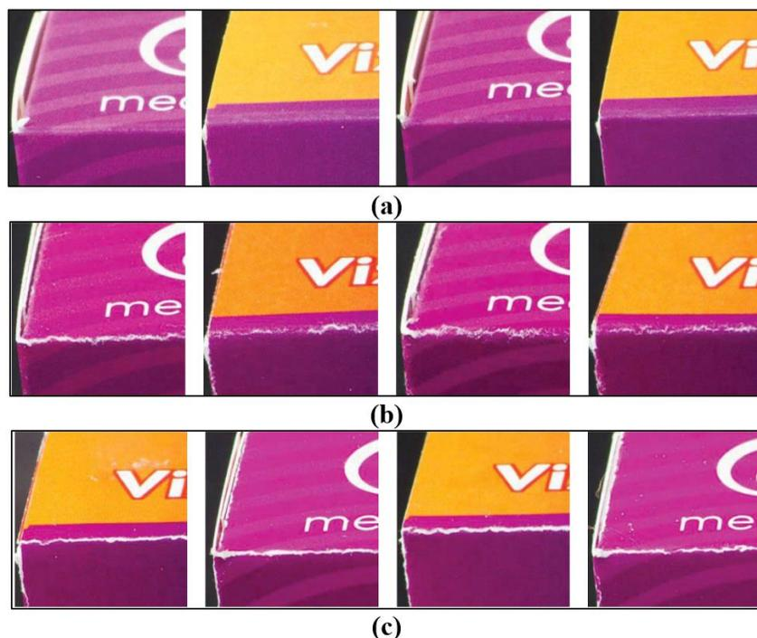
**Fig. 12.** Examples of paperboards after creasing and folding with: (a) good, (b) insufficient, and (c) poor cracking resistance. Reprinted with permission from Bota *et al.* (2022).
