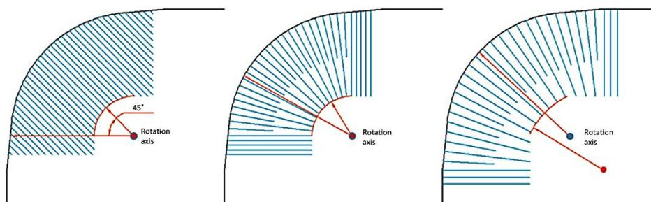
**Fig. 2.** Examples of creasing patterns available for production of paperboard tray blanks (Tanninen *et al.* 2015a).
