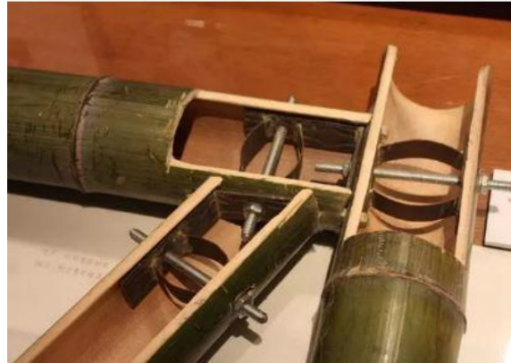
Fig. 5. Bolted joints examples from Hong et al. (2019); CC BY 4.0
