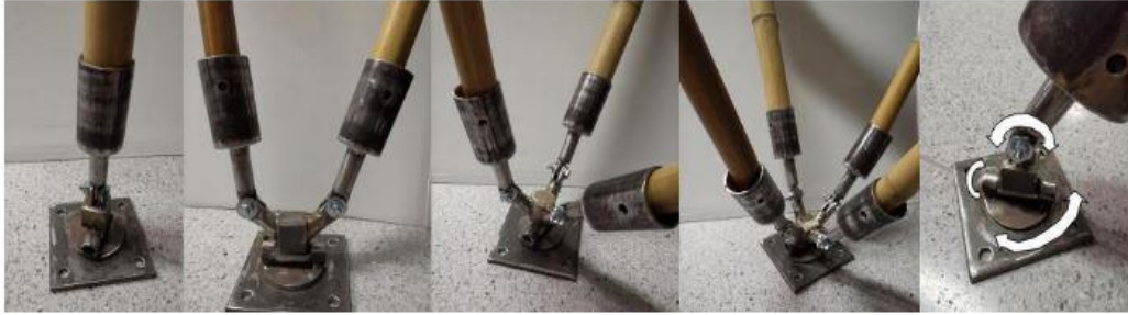
Fig. 7. Fit test between the metal and bamboo parts(Source: Rittironk 2021); CC BY-NC-ND 4.0
