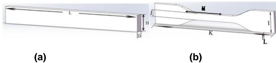
Fig. 3. Dimensions of composite specimens prepared for mechanical testing (a: bending strength, L=127 mm, H=12.7 mm, D=3.2 mm; a: impact strength, L=80 mm, H=10 mm, D=4 mm; b: tensile strength, K=115 mm, J=6 mm, L=3mm, M=25 mm, l=18 mm)
