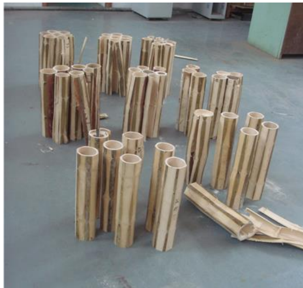
Fig. 14. Longitudinal compressive test results
