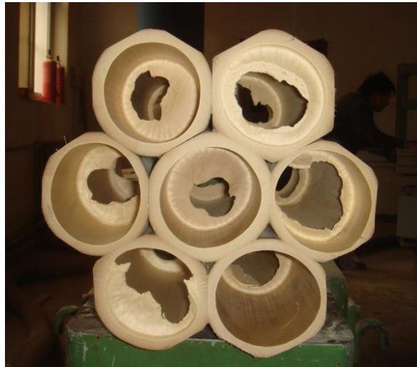
Fig. 5. Glued HexBam cross section diagram
