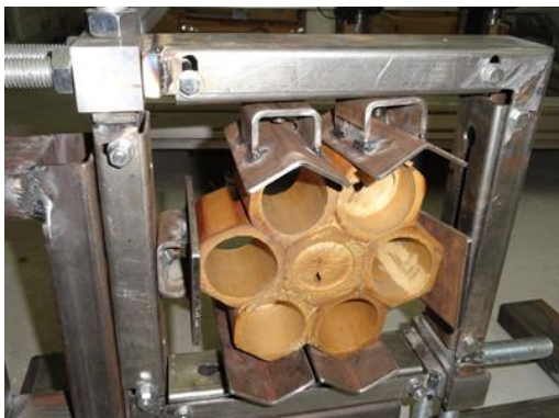
Fig. 3. The horizontal molding fixture
