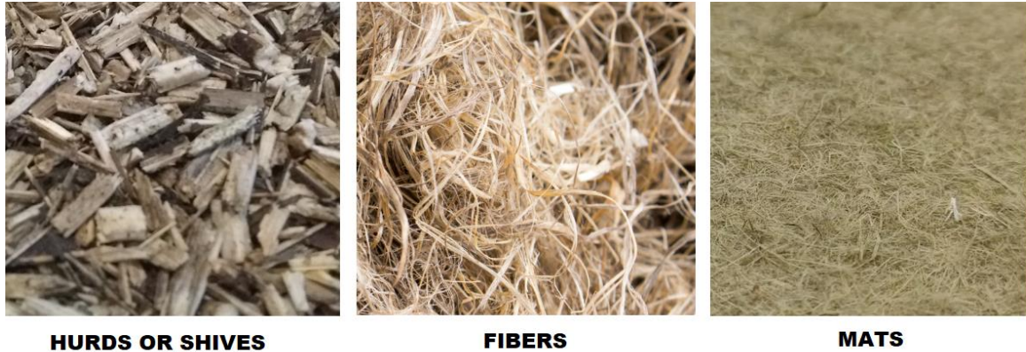
Fig. 2. Hemp by-products experimented as mycelium growth substrates
