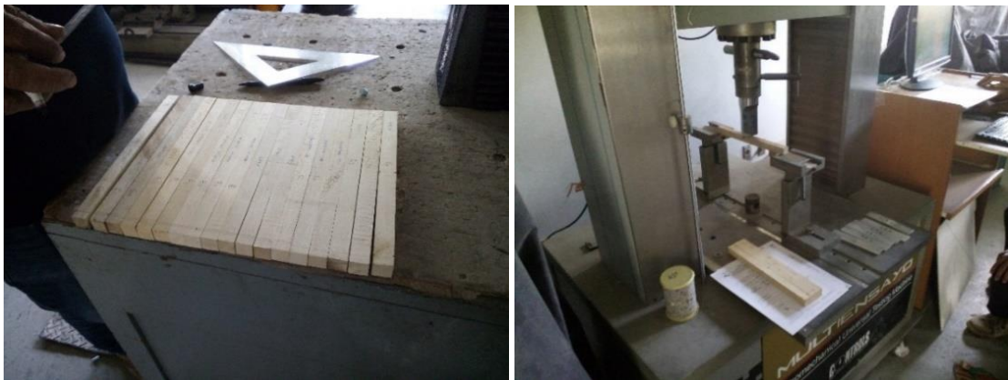
Fig. 2. One white jabon specimen being tested of its static bending using a universal testing machine (UTM)
