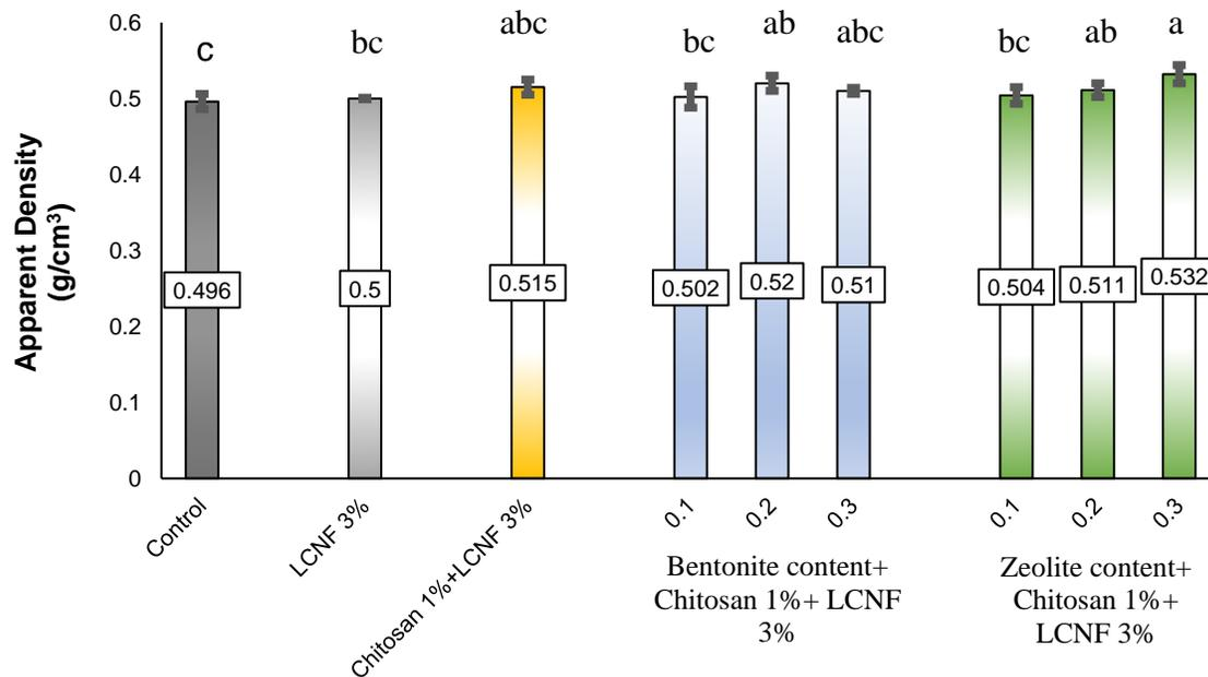
**Fig. 10.** The effect of treatments on apparent density of recycled paper. Plotted points that do not share the same letter were significantly different from each other (99% confidence level).
