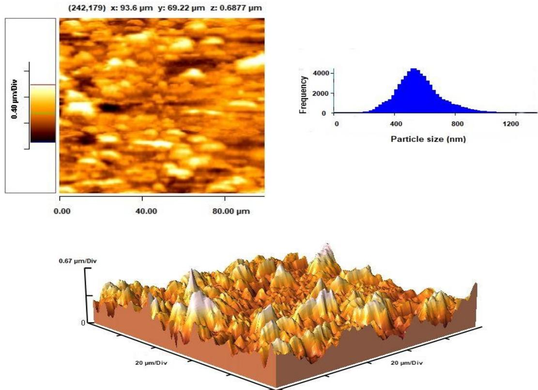
**Fig. 3.** Topography and dimensions of bentonite microparticle
