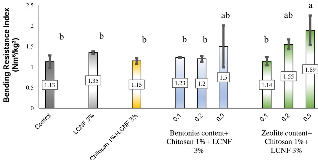
**Fig. 14.** The effect of treatments on bending resistance index of recycled paper. Plotted points that do not share the same letter were significantly different from each other (99% confidence level).
