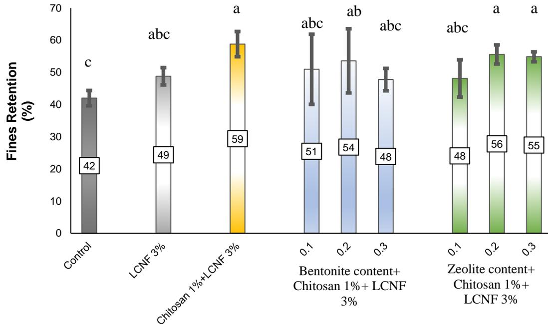
**Fig. 9.** The effect of treatments on fines retention of recycled pulp suspension. Plotted points that do not share the same letter were significantly different from each other (99% confidence level).
