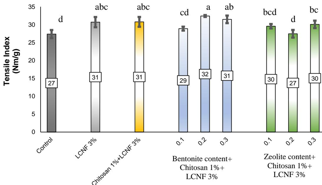
**Fig. 12.** The effect of treatments on tensile index of recycled paper. Plotted points that do not share the same letter were found to be significantly different from each other (99% confidence level).
