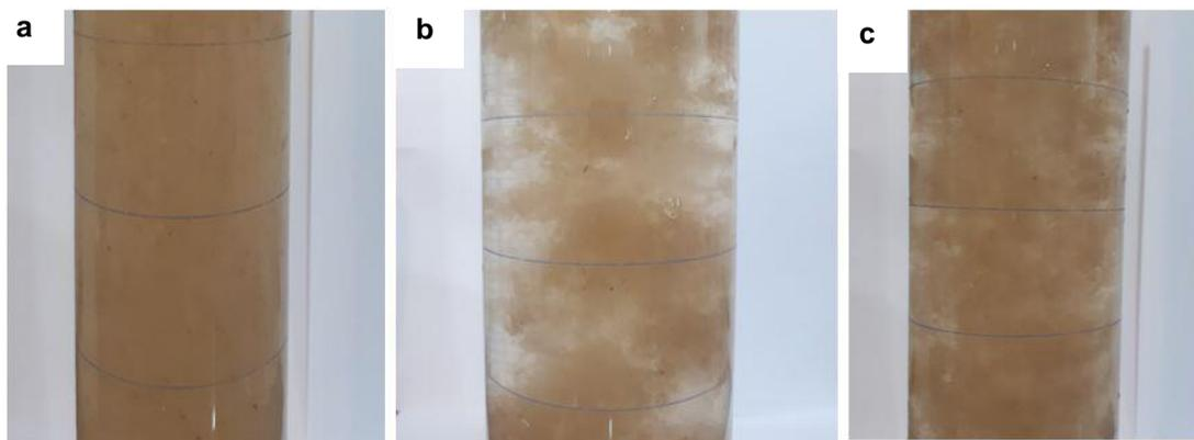
**Fig. 8.** Visualizing of flocculation phenomenon in: a: pulp containing LNFC, b: pulp containing LNFC only treated with 1% chitosan and c: pulp containing LNFC treated with 1% chitosan + 0.3% microparticle (zeolite).
