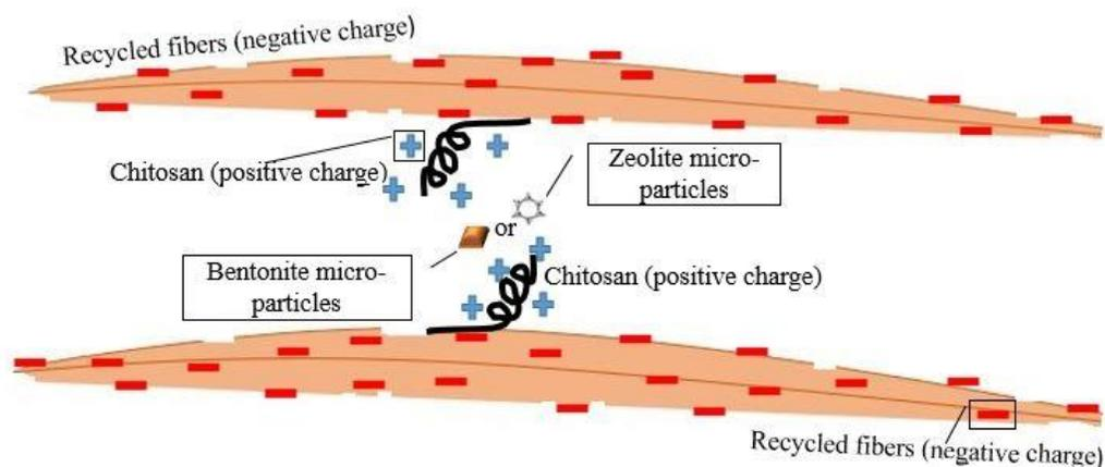
**Fig. 7.** Probable mechanism of floc formation with microparticle system
