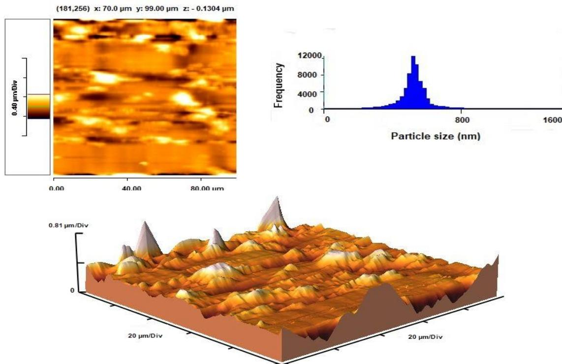
**Fig. 1.** Topography and size distribution of zeolite
