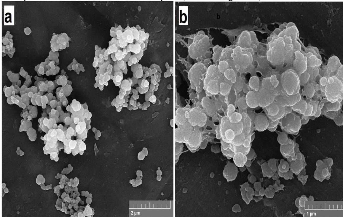
Fig. 2. FESEM images of zeolite microparticles
