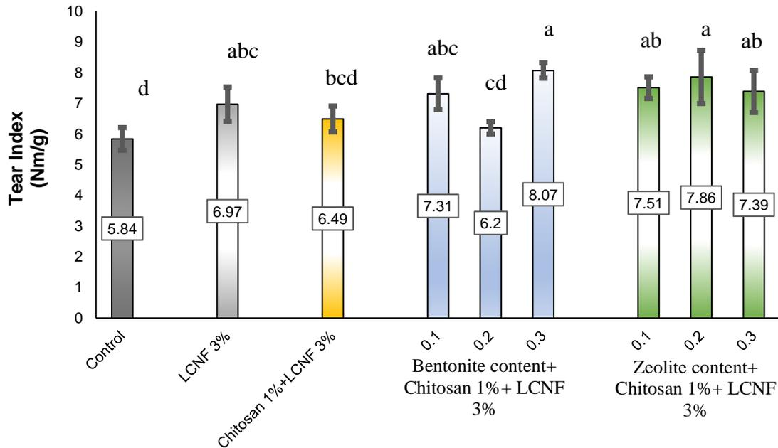
**Fig. 13.** The effect of treatments on tear index of recycled paper. Plotted points that do not share the same letter were significantly different from each other (99% confidence level).
