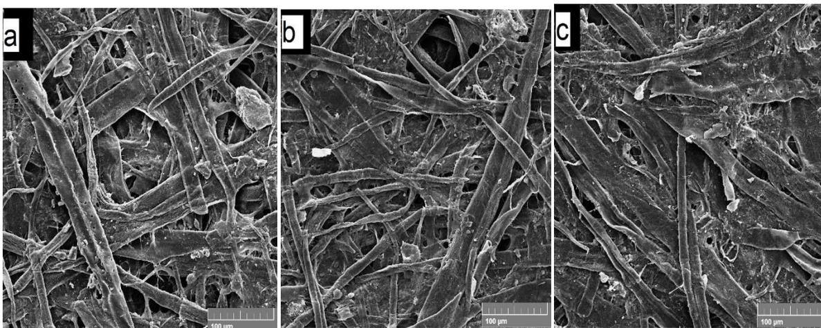
**Fig. 11.** FE-SEM images of made papers with: a) no additive (control), b) only 3% LNFC, c) 3% LNFC+1% chitosan +0.3% zeolite.
