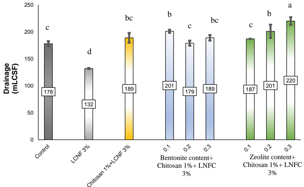
**Fig. 6.** Effect of treatments on drainage of recycled pulp suspension. Plotted points that do not share the same letter were found to be significantly different from each other (99% confidence level)
