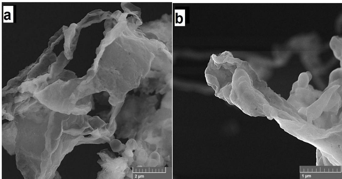
**Fig. 4.** FESEM images of bentonite microparticles (overlapped bentonite platelets)
