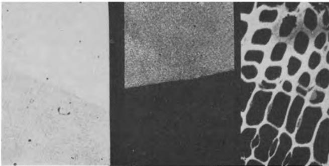
**Fig. 25** — A microradiogram of *Picea excelsa* and the corresponding step wedge
