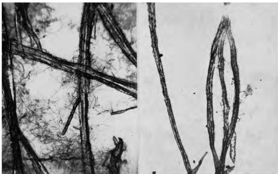
Fig. 21—Normal wood fibres from Pinus radiata prepared by the sulphate process and beaten in the Lampen mill for 72 min. ( \times 120 )—note swelling and development of external fibrillation
