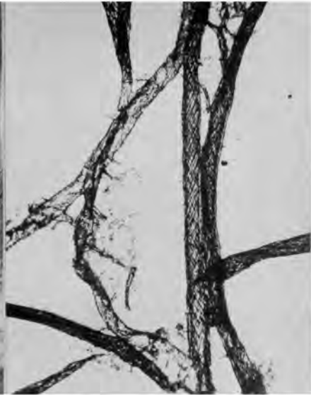
Fig. 7. —Compression wood fibres as observed in pulp prepared from Pinus radiata compression wood ( \times 110 )—note the characteristic striations
