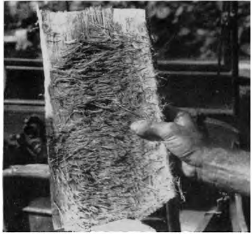
Fig. 3 —An example of the excessive 'woolliness' that is encountered on the sawing of logs containing bands of tension wood
