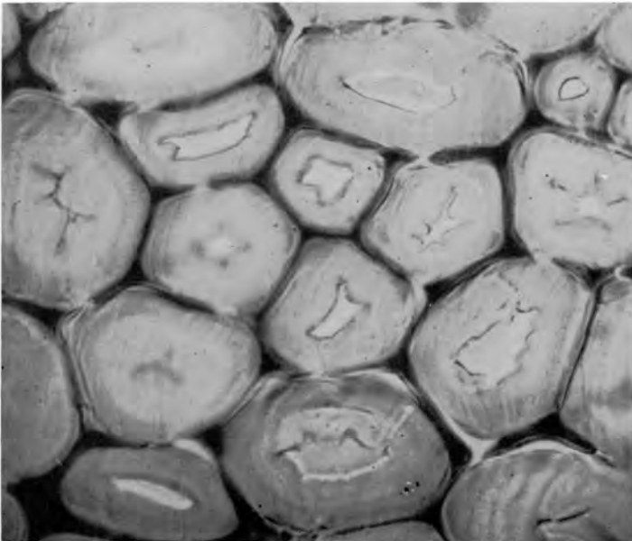
Fig. 19—Cross-section of tension wood from Eucalyptus elaeophora taken in ultra-violet light—note heavy absorption in the intercellular zone and the weak absorption in the cell wall, particularly in the layer G ( \times 2\ 000 )
