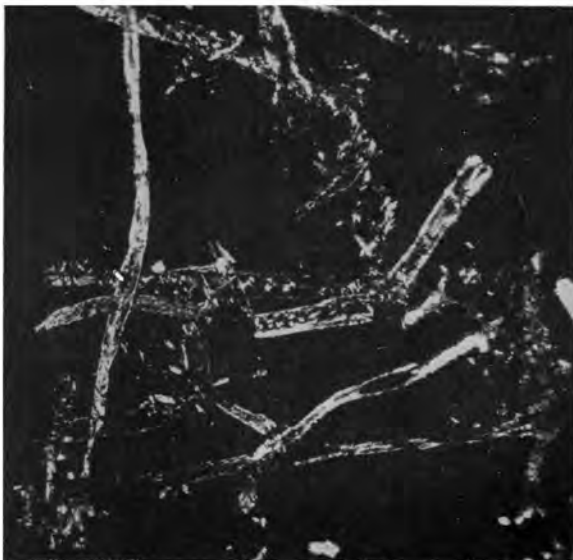
Fig. 24—Pulp prepared by the sulphite process from the heartwood zone of the log illustrated in Fig. 1, photographed between crossed nicols ( \times 65 )—note number of broken fibres
