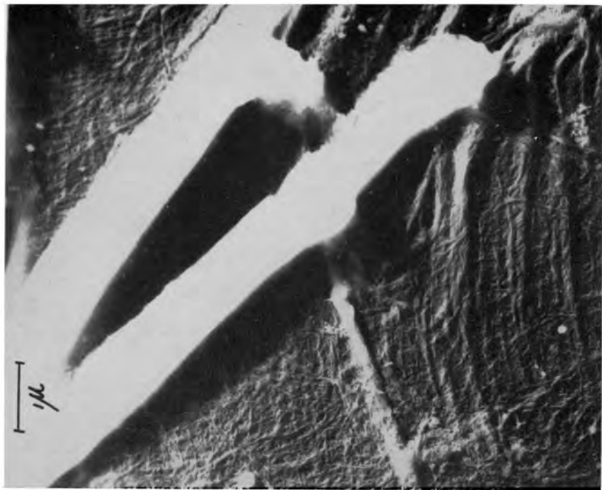
Fig. 14—Electron micrograph of a delignified longitudinal section of a compression wood tracheid of Pinus radiata showing two displaced parts of the helically wound layer S2 overlying the layer S1 (uranium-shadowed) (cf. Fig. 12)
