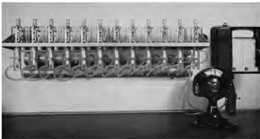
Fig. 17 — Apparatus for the study of hygro- and hydrostability
