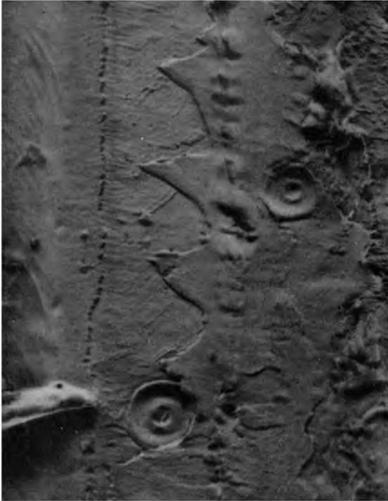
**Fig. 18** — Radial surface of European spruce near middle lamella (metal shadowed plastic solid replica  $\times 750$ )
