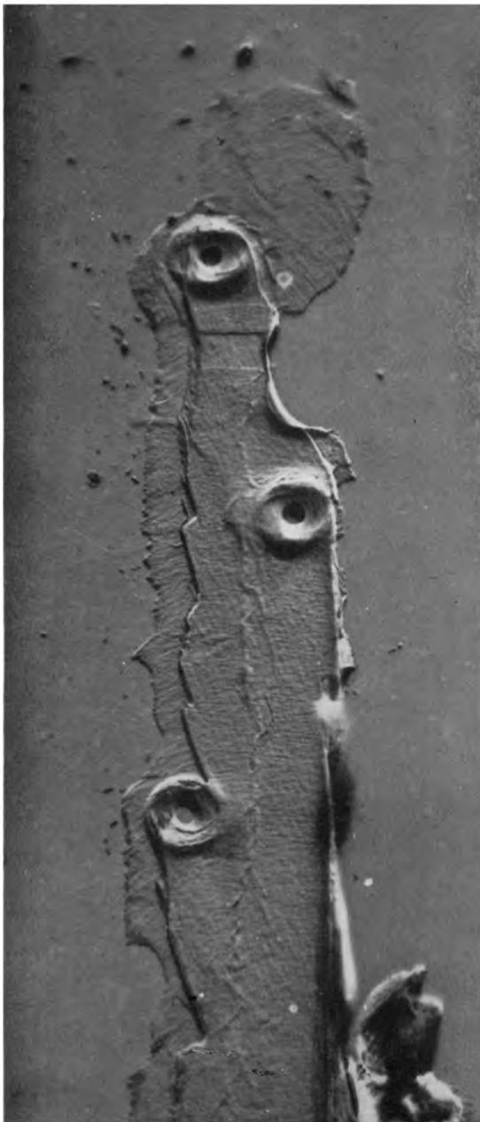
**Fig. 16** — Macerated Scots pine — S3 overlies S2, the fracture line of which may be seen sweeping round the pits
