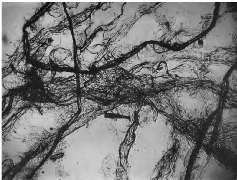
Fig. 2 — Fibrillation by ultrasonic treatment, according to Algar and Giertz (5) — (a) Spruce sulphate fibre
