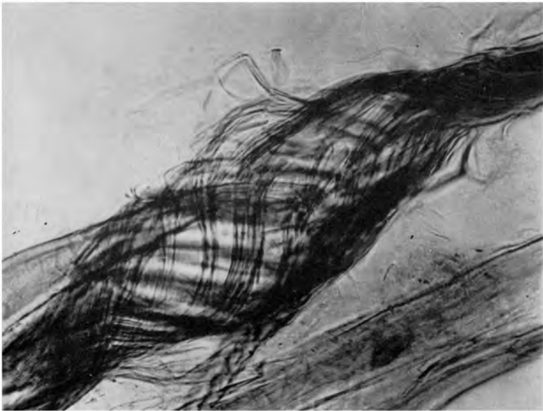
Fig. 2 — Fibrillation by ultrasonic treatment, according to Algar and Giertz (5) — (b) Soft sulphite pulp
