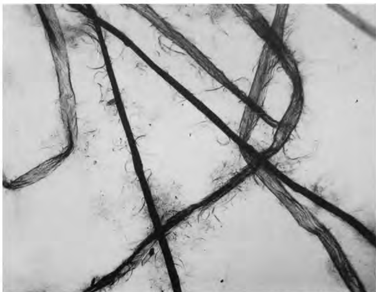
Fig. 2 — Fibrillation by ultrasonic treatment, according to Algar and Giertz (5) — (c) Kraft pulp
