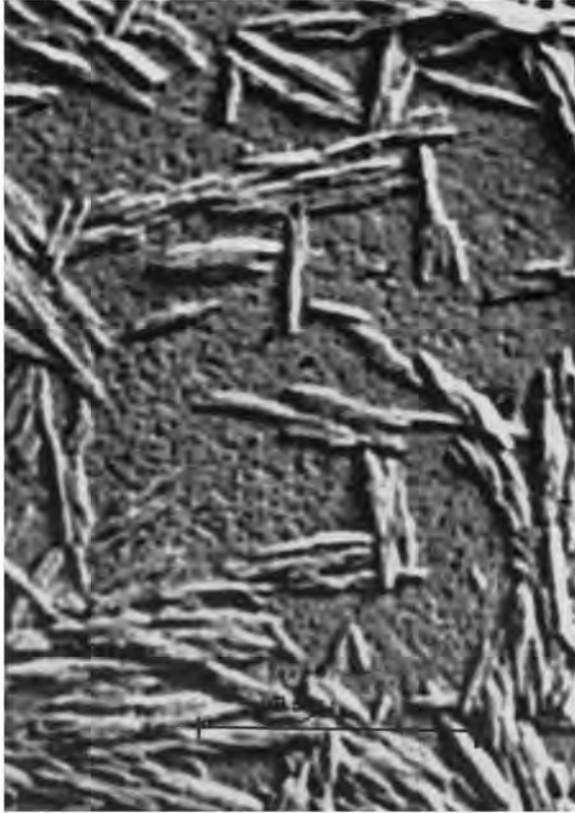
Fig. 11 —Micelles from hydrolysed native ramie fibres, deposited on a glass surface, shadowed with palladium at an angle ( \theta ) with \text{tg}\theta=0.2 , from Morehead ( unpublished ) (magnification \times 47\ 000 )
