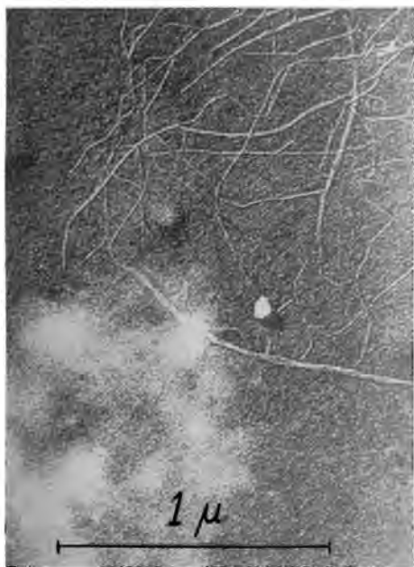
Fig. 9—Electron micrograph of holocellulose from spruce, dispersed by ultrasonic irradiation, showing cellulose fibrils and 'clouds' of hemicellulose, from Rånby (17) (magnification \times 40\,000 )
