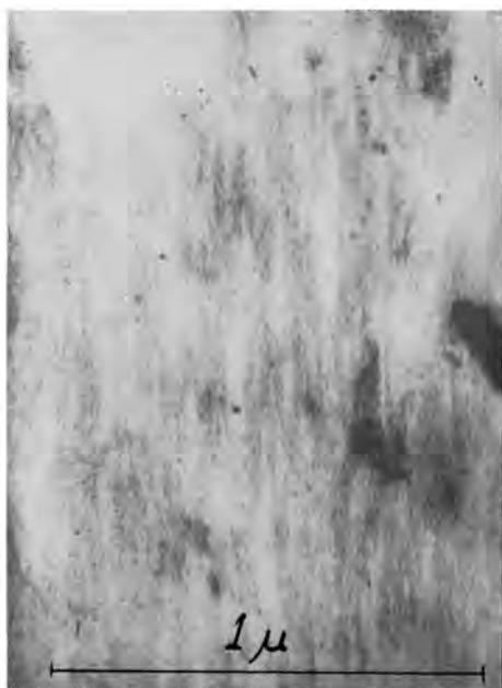
Fig. 10—A section of an aspen wood fibre (parallel with the fibre axis) stained with thallium ethylate, from Asunmaa (16) (magnification \times 52\,000 )
