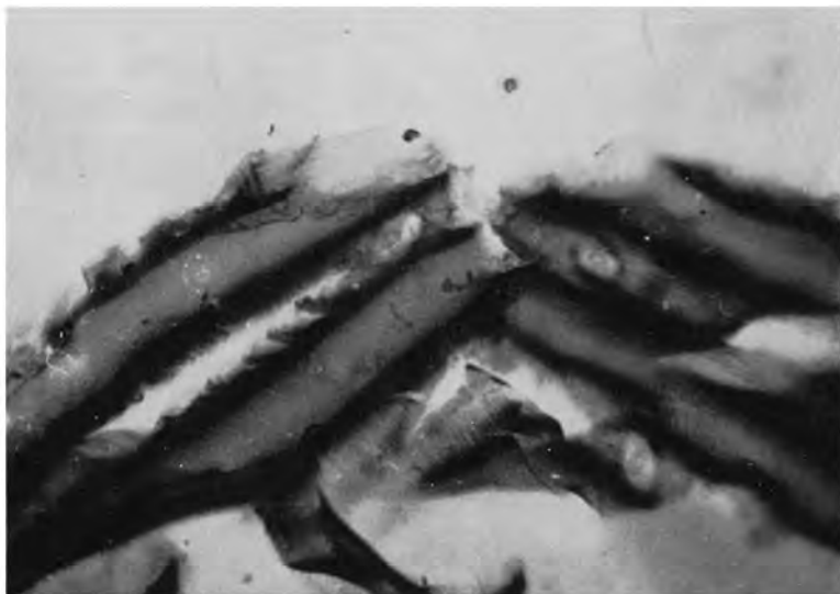
Fig. E —The primary wall from a strong sulphite fibre after the secondary wall has been dissolved in cuprammonium solution — note the dark longitudinal formations that originate from the middle lamella and the torus fixed on the membrane in the pit opening
