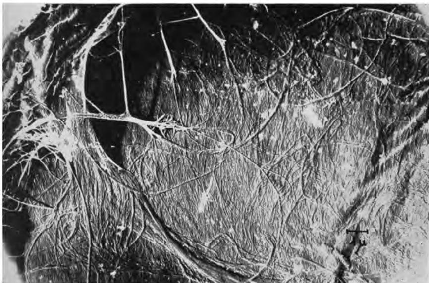
**Fig. 24**—Lamella of the outer secondary wall of the upper fibre forms a fibre bond in a pine kraft pulp
