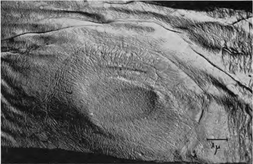
**Fig. 19**—Pit membrane in a sulphite pulp having dried on to the collapsed pit yard and the tertiary wall opposite—no striking drying features are visible
