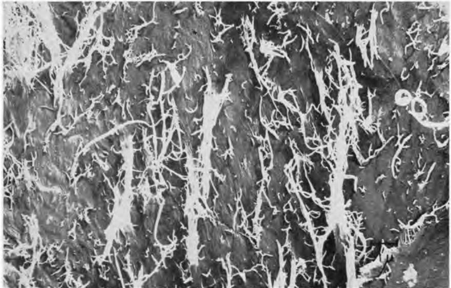
**Fig. 28**—Former area of contact between two fibres in a spruce sulphite pulp, made visible by tearing apart the formerly bonded fibres
