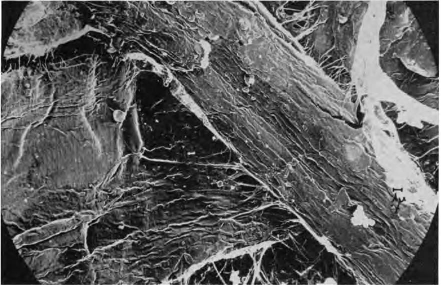
**Fig. 13**—Uncollapsed late wood cell crossing a collapsed early wood cell in a technical printing paper
