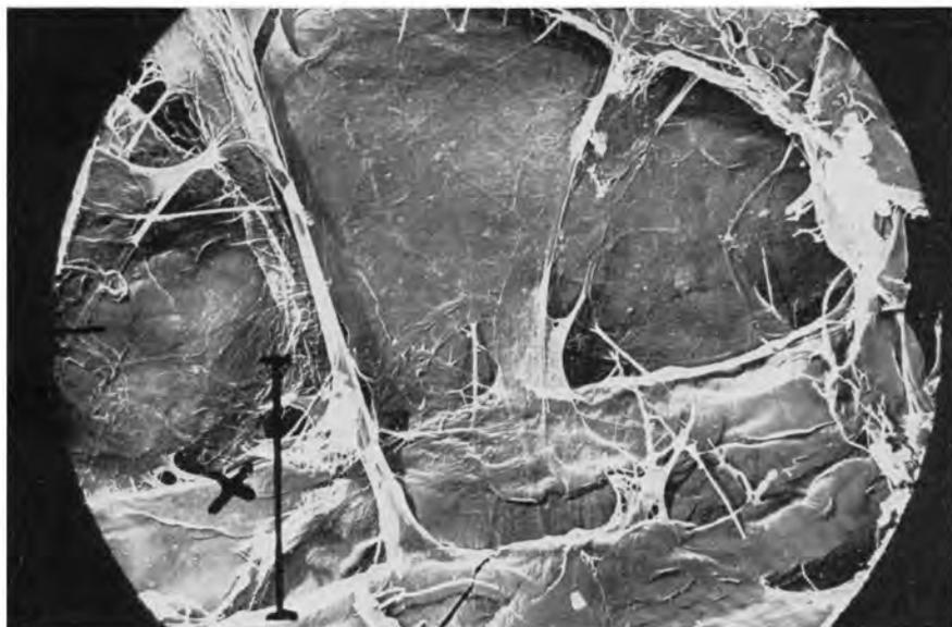
**Fig. 29**—Various fibre bonds in a pine kraft pulp
