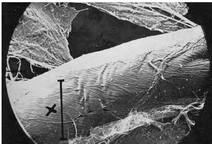
**Fig. 12**—Compression wood cell in a coniferous wood pulp
