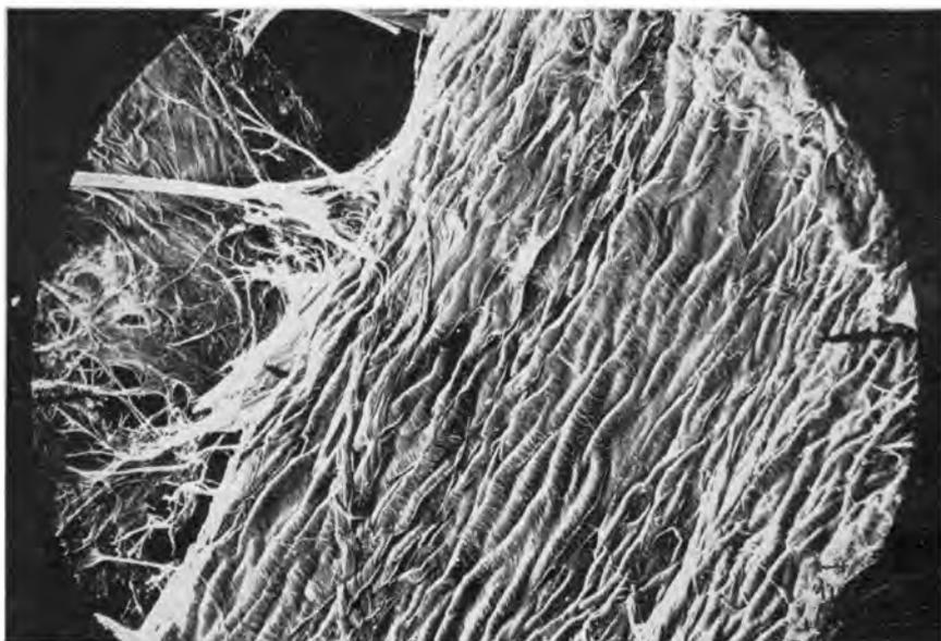
**Fig. 16**—Pulp fibre in a technical filter paper that has been treated with alkali—the outer secondary wall has become too large for the extracted inner layers and, after drying, shows many axially running wrinkles
