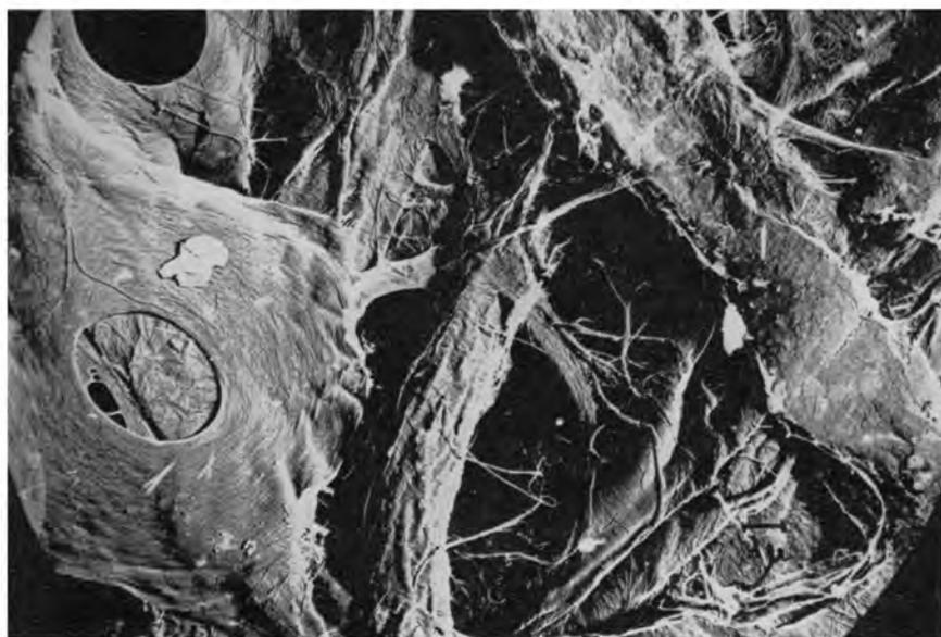
**Fig. 32**—Part of a pine pulp sheet showing bonded fibre fragments
