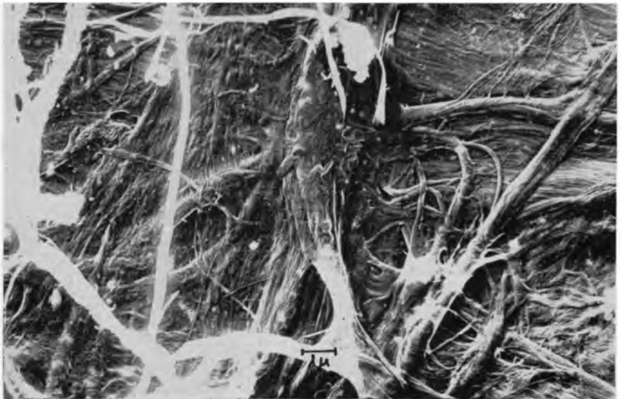
**Fig. 38**—High disorder of formerly textured fibre wall remnants—the pulp sheet loses the character of a fibre sheet
