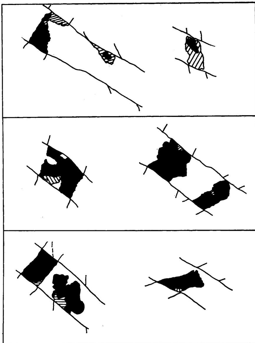
Fig. 7—Fields illustrating (above) stress-relieving, (centre) non-stress-relieving and (below) possible stress-relieving bond breakage—the hatched regions indicate breakage, the black regions residual bond
