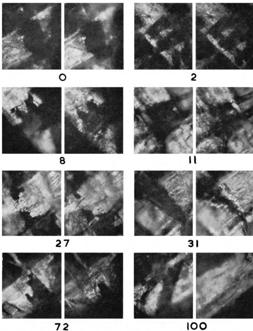
**Fig. 1**—A selection of fields showing bond breakage after tensile straining—figures indicate the percentage breakage
