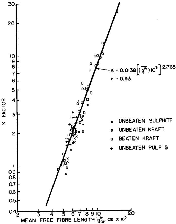
Fig. 6—Relationship between  $K$  factor and mean free fibre length
