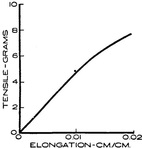
Fig. 4—Stress/strain curve of a single fibre (spruce sulphite pulp—1 000 lb/in<sup>2</sup> pressure)
