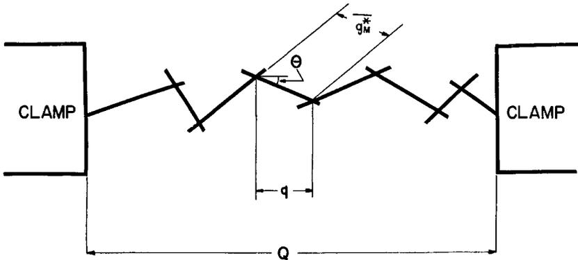
Fig. 3—Chain of free fibre lengths
