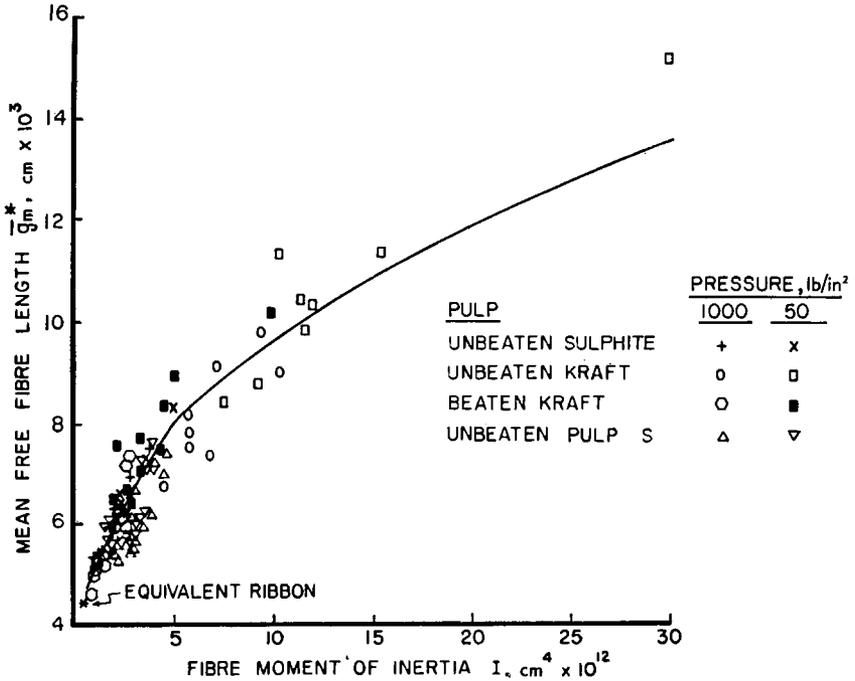
Fig. 5—Relationship between 'fibre moment of inertia' and mean free fibre length
