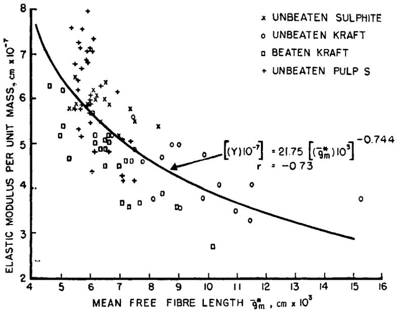
Fig. 7—Relationship between elastic modulus per unit mass and mean free fibre length
