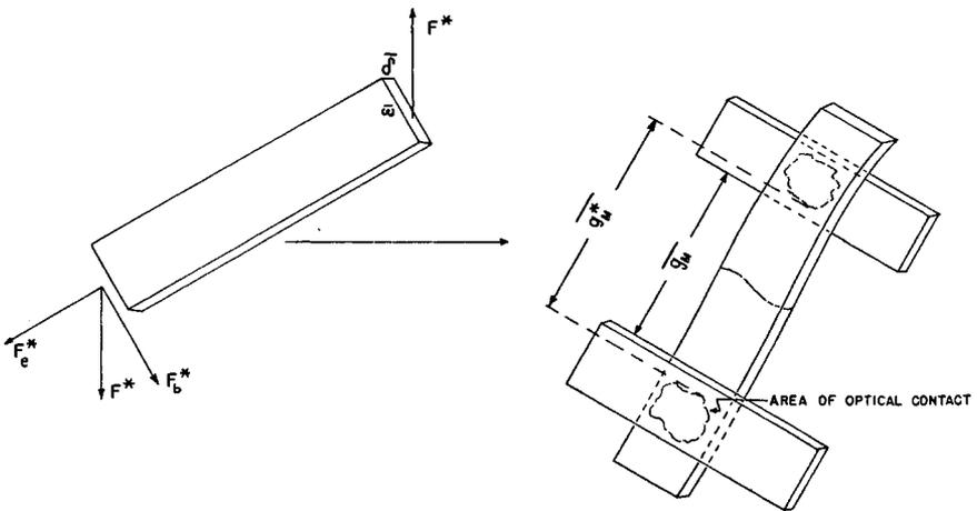
*Fig. 1*—Distortion of free fibre length during straining (exaggerated for demonstration purposes)
