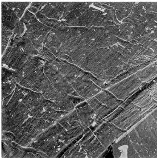
Fig. 4—(Above) Wrinkles (microcompressions) in a fibre produced by enforced longitudinal shortening when dried on cellulose film ( \times 180 )
