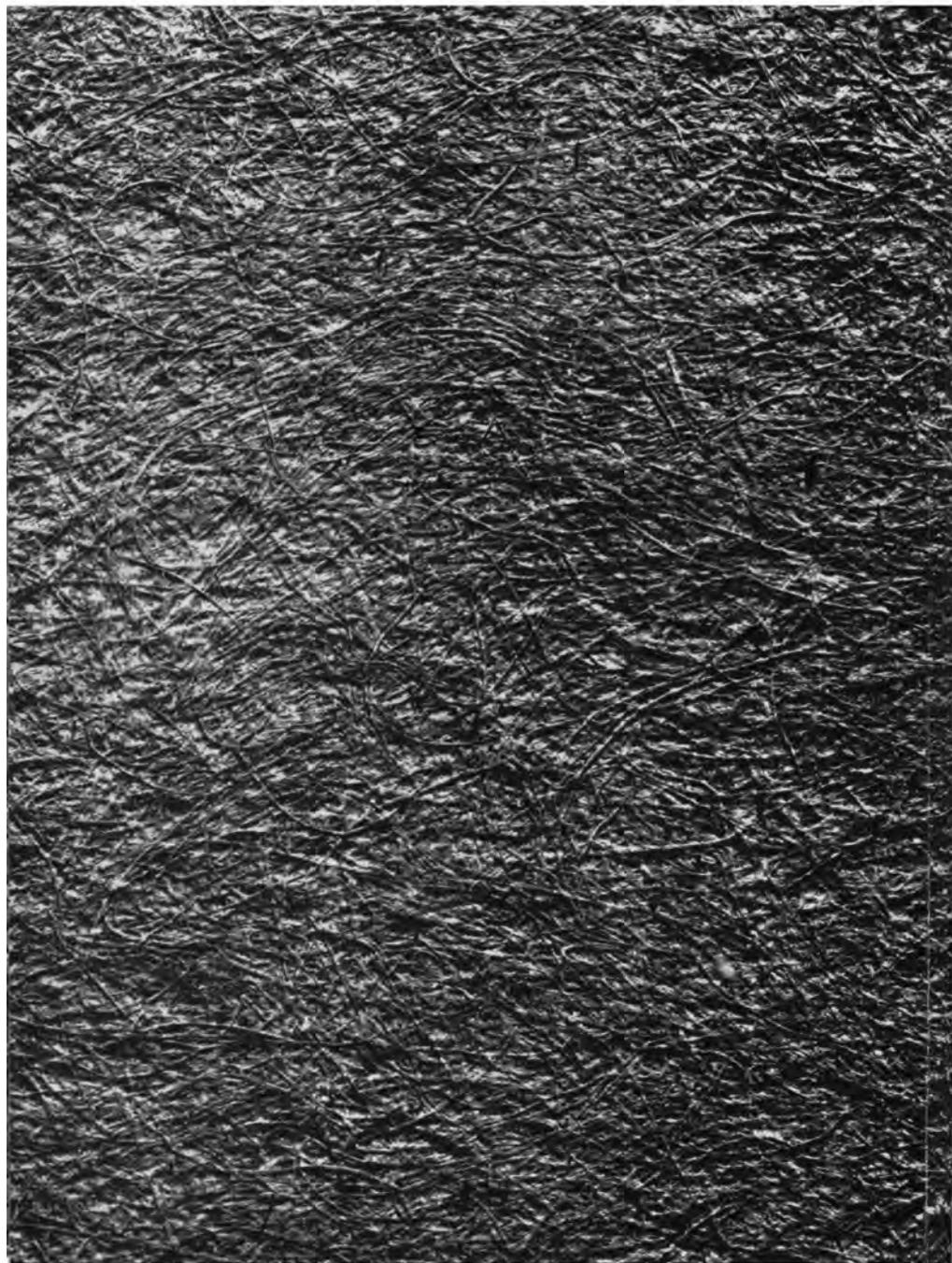
**Fig. 32**—Kraft paper—a clear impression of the preferred orientation of fibres in the machine-direction (across the micrograph) is given at this low power ( $\times 20$ )
