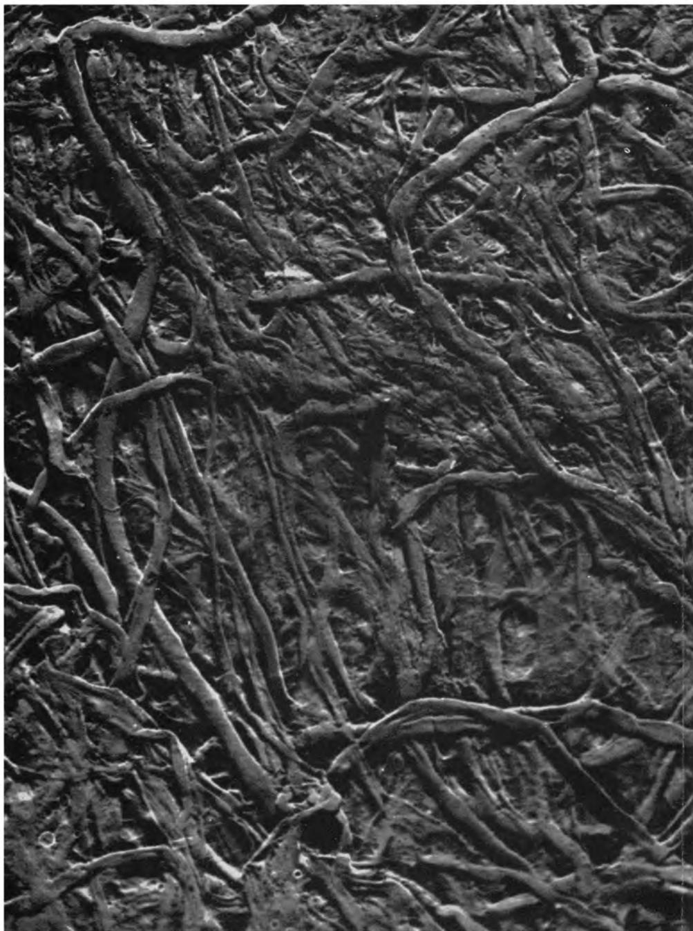
**Fig. 27**—Effect of watermarking on £1 Bank of England note—The prominent watermark is seen as a depression of the surface running from centre left to the lower right corner ( $\times 275$ )
