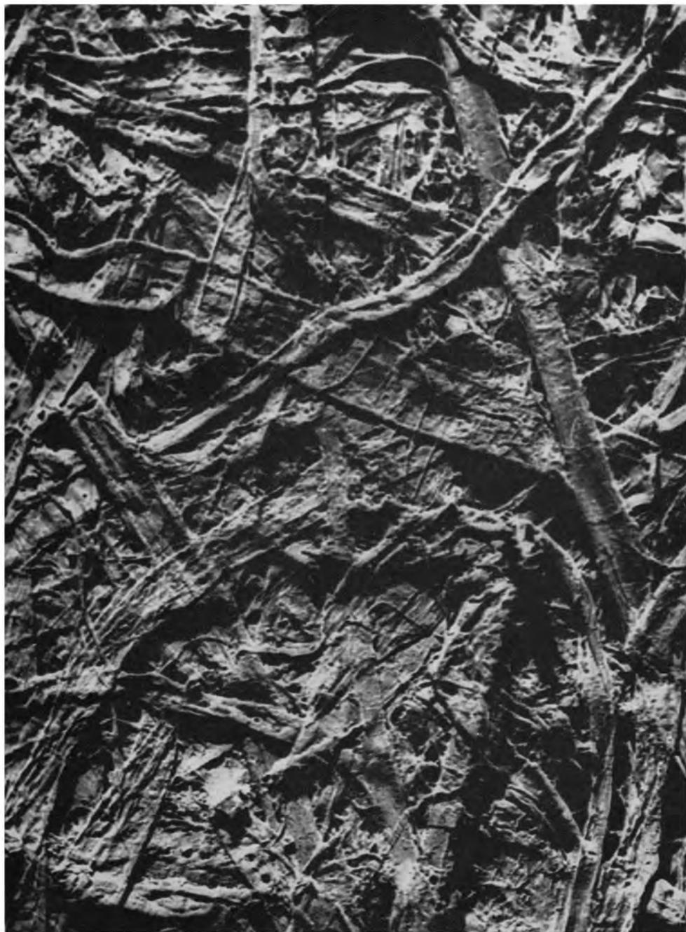
**Fig. 11**—Mechanical printing, wire side, before supercalendering ( $\times 275$ )
