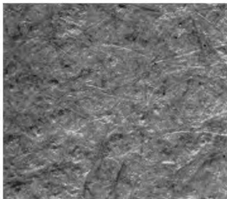
*Fig. D3a*—Surface detail after moderate laboratory supercalendering
