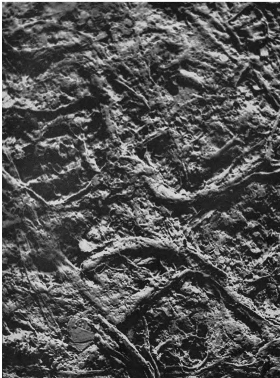
**Fig. 25**—Unsatisfactory mechanical printing
