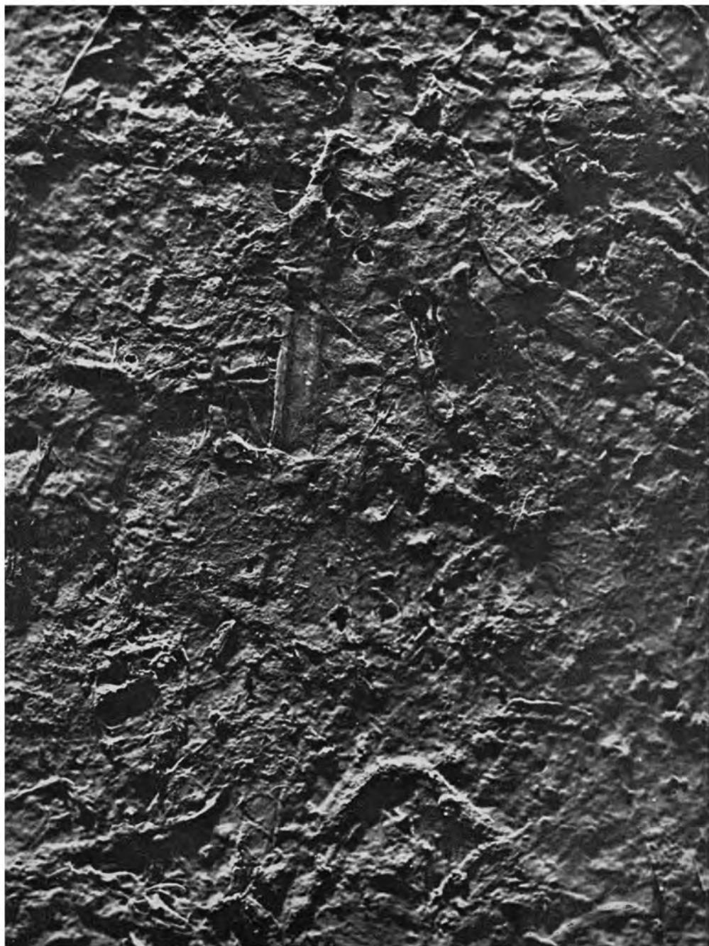
**Fig. 5**—Greaseproof, top side**( $\times 275$ )**
