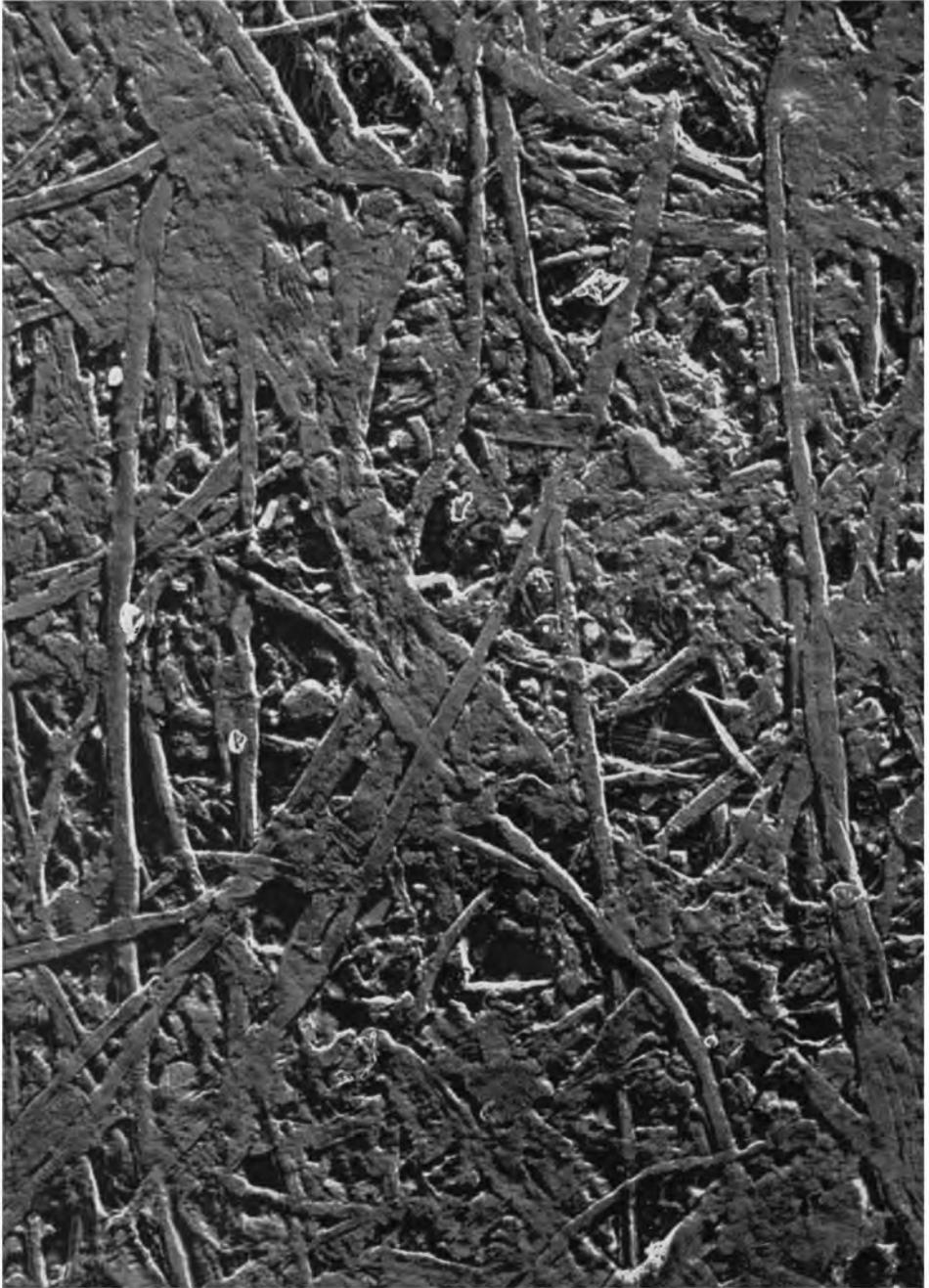
**Fig. 30**—Imitation art paper—the esparto furnish, the heavy clay loading and the effect of supercalendering are apparent ( $\times 275$ )
