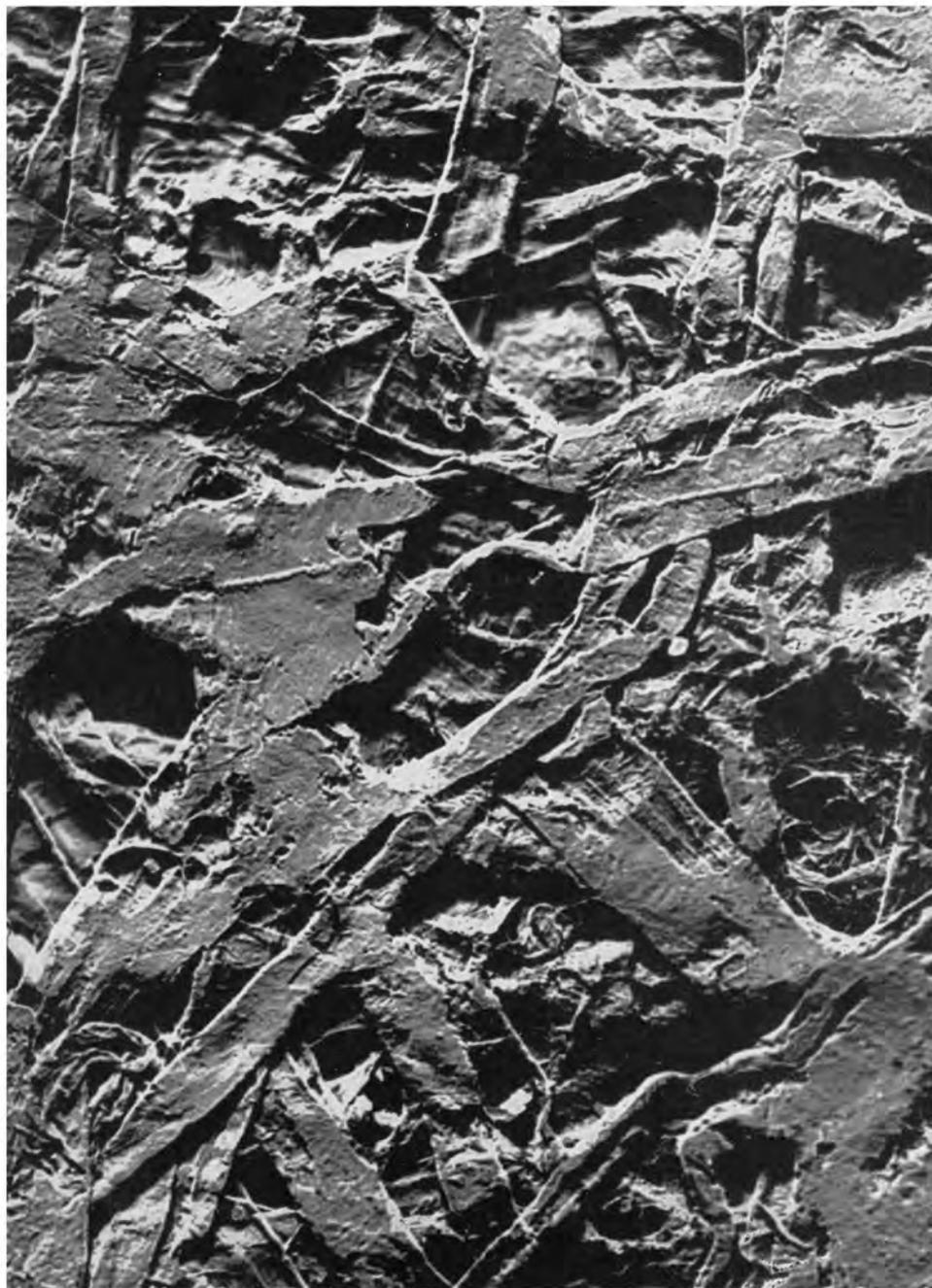
*Fig. 15*—Machine-glazed kraft paper, wire side
