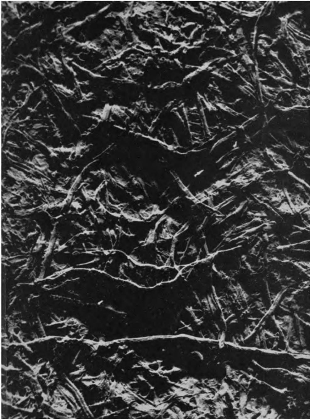
**Fig. 31**—Drawing paper—a hand-made sheet with 100 per cent rag furnish [The comparative roughness of the surface is indicated by the long shadows] ( $\times 110$ )
