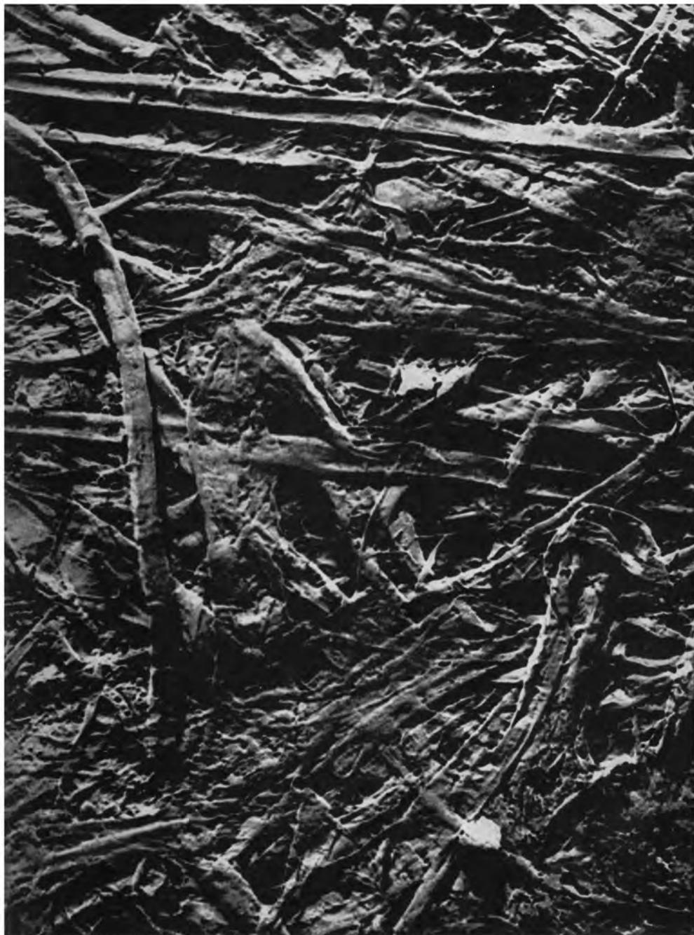
**Fig. 12**—Mechanical printing, wire side, after supercalendering (× 275)
