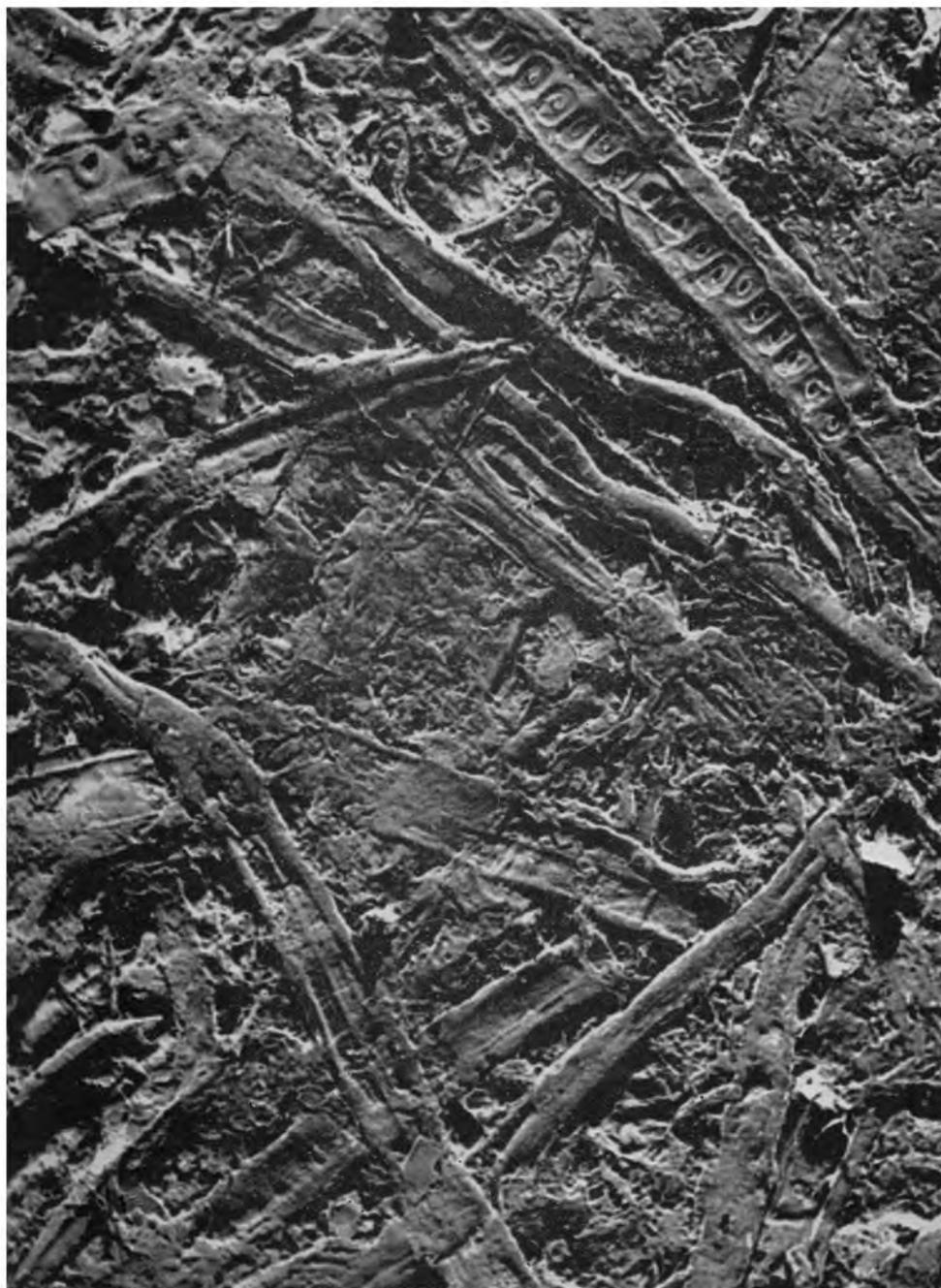
*Fig. 10*—Mechanical printing, top side, after supercalendering ( $\times 275$ )
