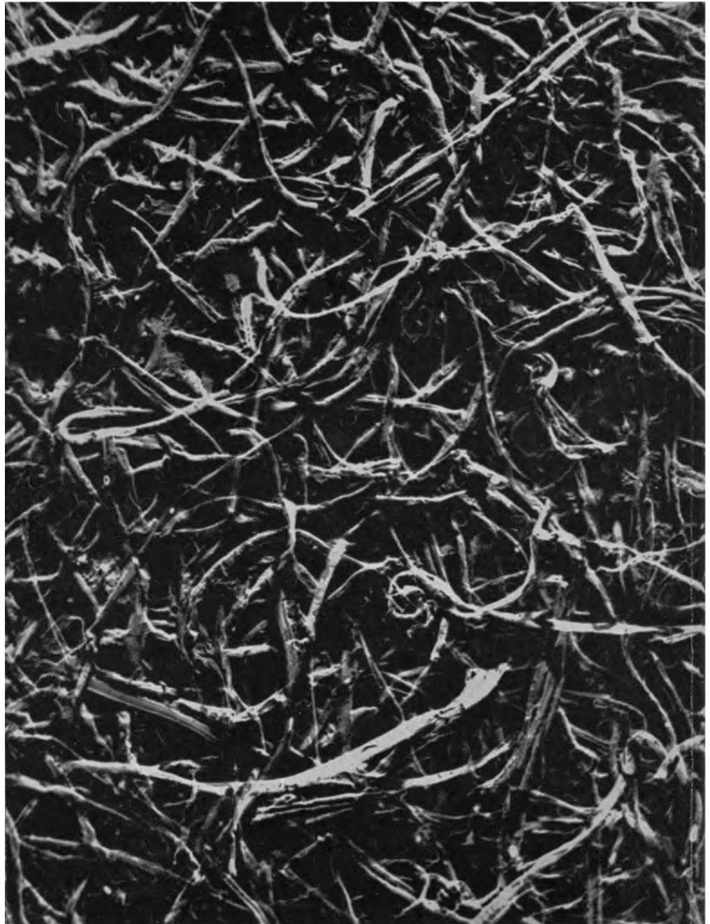
**Fig. 34**—Blotting paper—the loose absorbent structure is strikingly revealed ( $\times 110$ )
