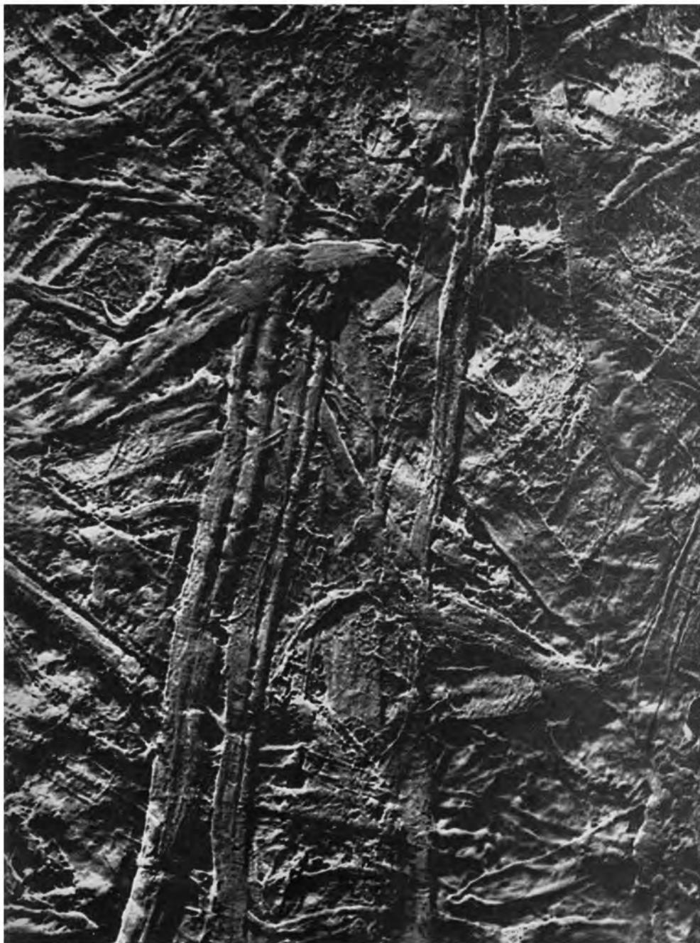
**Fig. 14**—Glazed imitation parchment, wire side, after supercalendering ( $\times 275$ )
