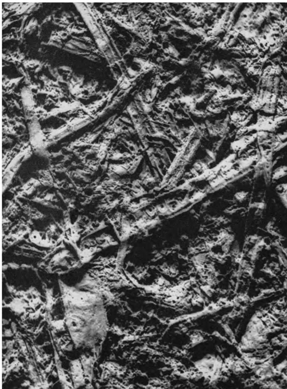
**Fig. 9**—Mechanical printing, top side, before supercalendering ( $\times 275$ )
