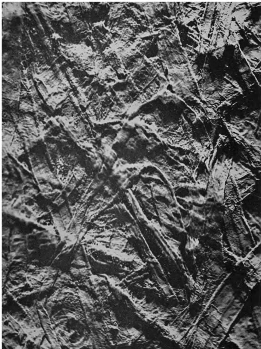
**Fig. 13**—Glazed imitation parchment, wire side, before supercalendering ( $\times 275$ )
