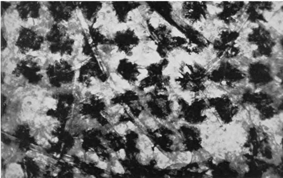
**Fig. 24**—Half-tone dot pattern on two mechanical printing papers ( $\times 90$ )
