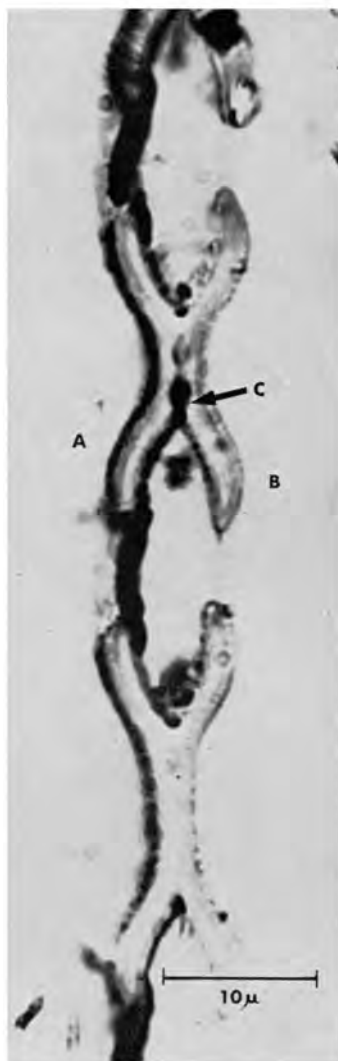
Fig. 13 —A tangential-longitudinal section of heartwood of P. radiata cut from a block stained by the Coppick and Fowler method, using the apparatus shown in Fig. 4(c): note the penetration of the cell A , the heavy staining of the torus and penetration of the reagents into the pit chamber (for further description, see text)
