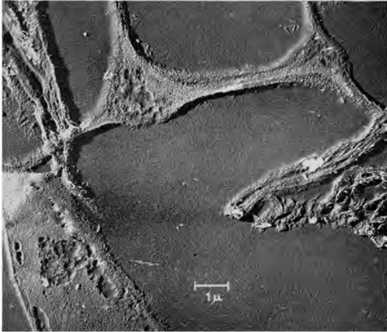
Fig. 15 —An electron micrograph of a section from a commercial sulphite pulp, showing the presence of unreacted corner thickenings
