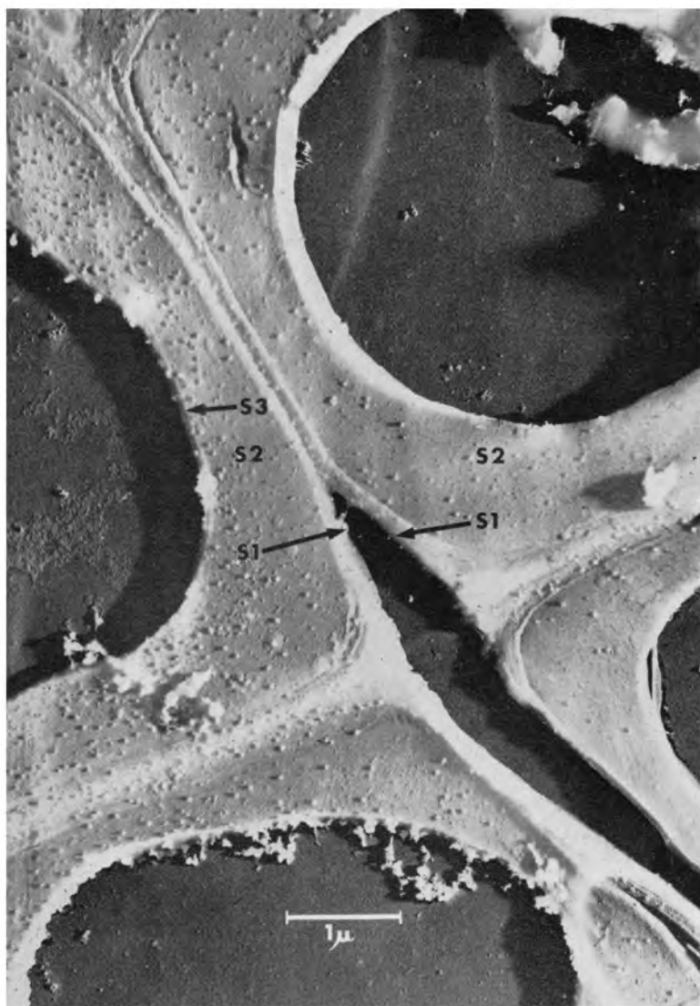
Fig. 10 —An electron micrograph of a transverse section of E. regnans after treatment with 6 per cent sodium hydroxide for 5 min at 100°C: note the separation in the middle lamella
