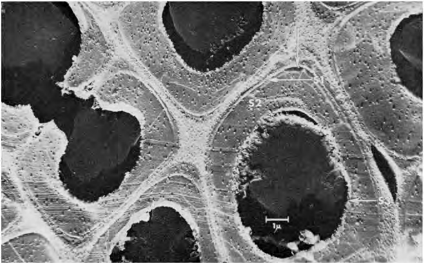
Fig. 12 —Similar to Fig. 10 and 11, showing incipient separation between the layers S1 and S2 (arrow)
