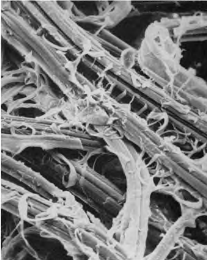
Fig. 3 —Electron micrograph of the surface of a sheet formed from fibrillated rayon ( \times 1\ 260 )
