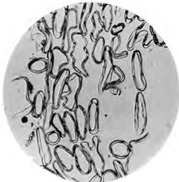
Fig. 1 —Cross-sections of wet hollow filament rayon fibres: the fibres were mounted for sectioning by embedding an oriented wet web in methyl methacrylate containing a water soluble plasticiser (methyl phthalyl ethyl glycollate) and carrying out a polymerisation according to Moore et al. (6) ( \times 245 )
