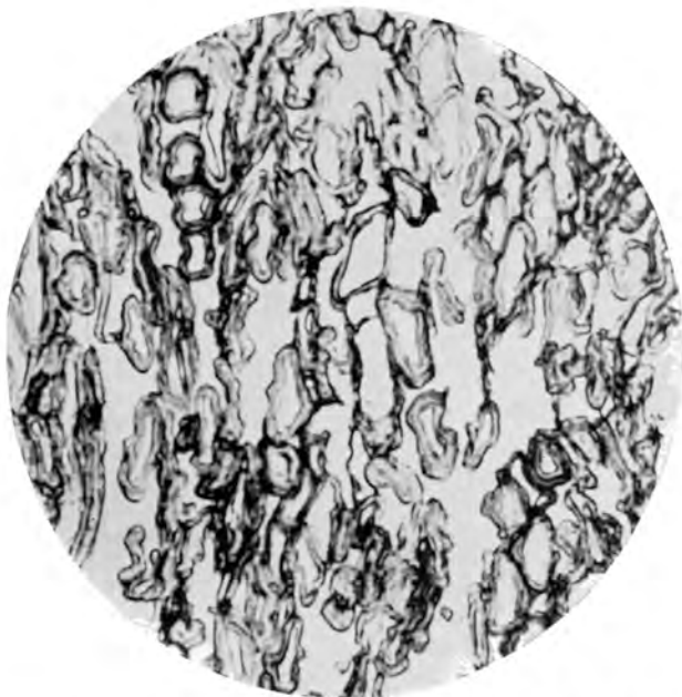
Fig. 7 —Cross-sections of high yield fibres (Fig. 5), after forming a sheet and drying ( \times 245 )
