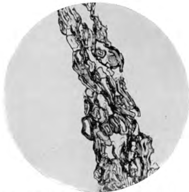
Fig. 8 —Cross-sections of low yield fibres (Fig. 6) after forming a sheet and drying ( \times 245 )
