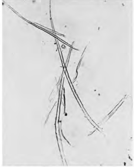
(h) Eucalyptus regnans holocellulose, beaten 10 min in M.S.E. homogeniser, unsilvered ( \times 90 )
