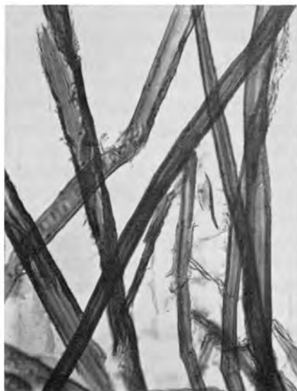
(a) Unbeaten Pinus radiata holocellulose, lightly silvered ( \times 140 )
