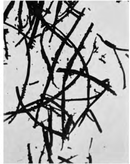
(j) Eucalyptus regnans holocellulose, beaten 10 min in M.S.E. homogeniser, heavily silvered ( \times 90 )
