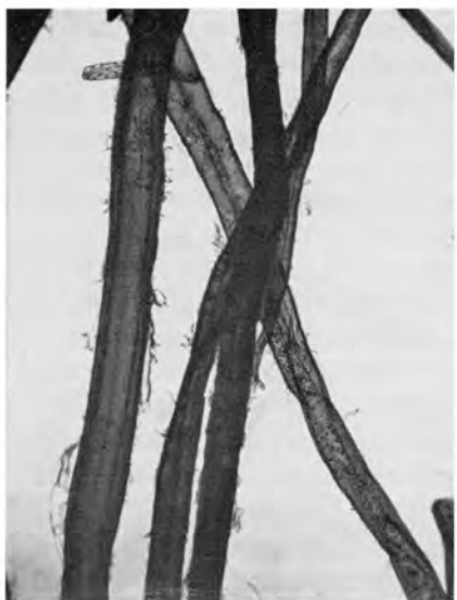
(c) Unbeaten spruce sulphite pulp, lightly silvered ( \times 140 )
