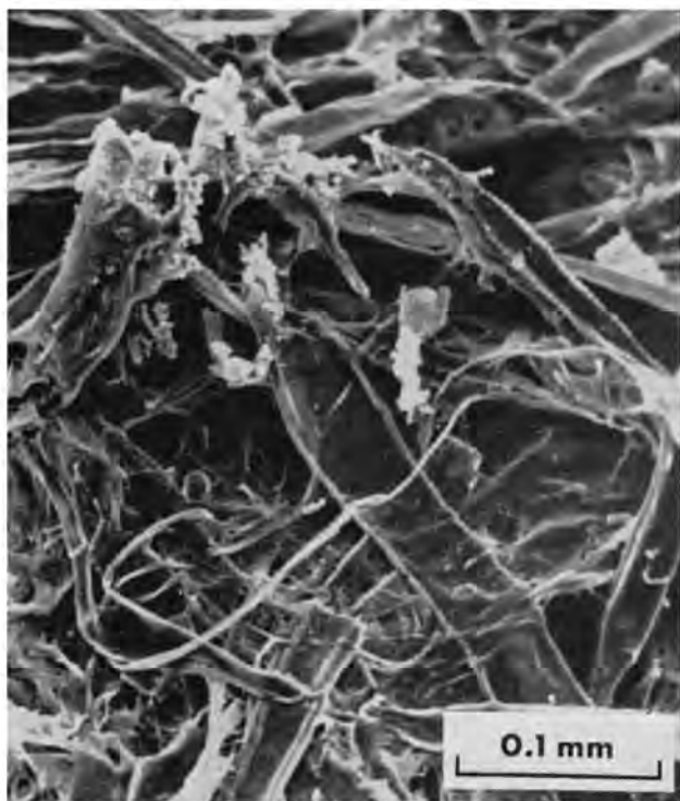
Fig. 9 —Raised mound of fibres on the wire side of an unpressed pulp pad made on a sheetmachine fitted with a Fourdrinier wire
