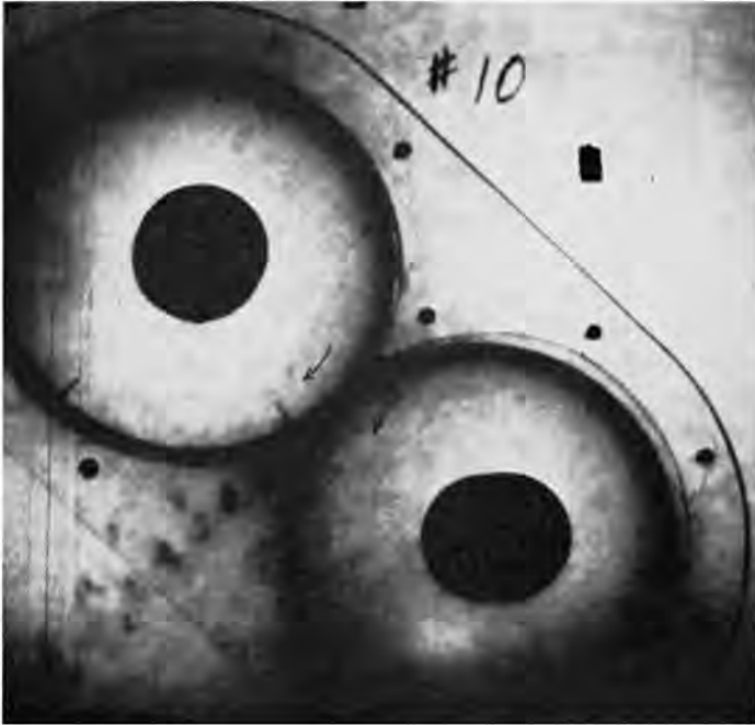
Fig. 4 —Still photograph showing formation of lumps by holey rolls
