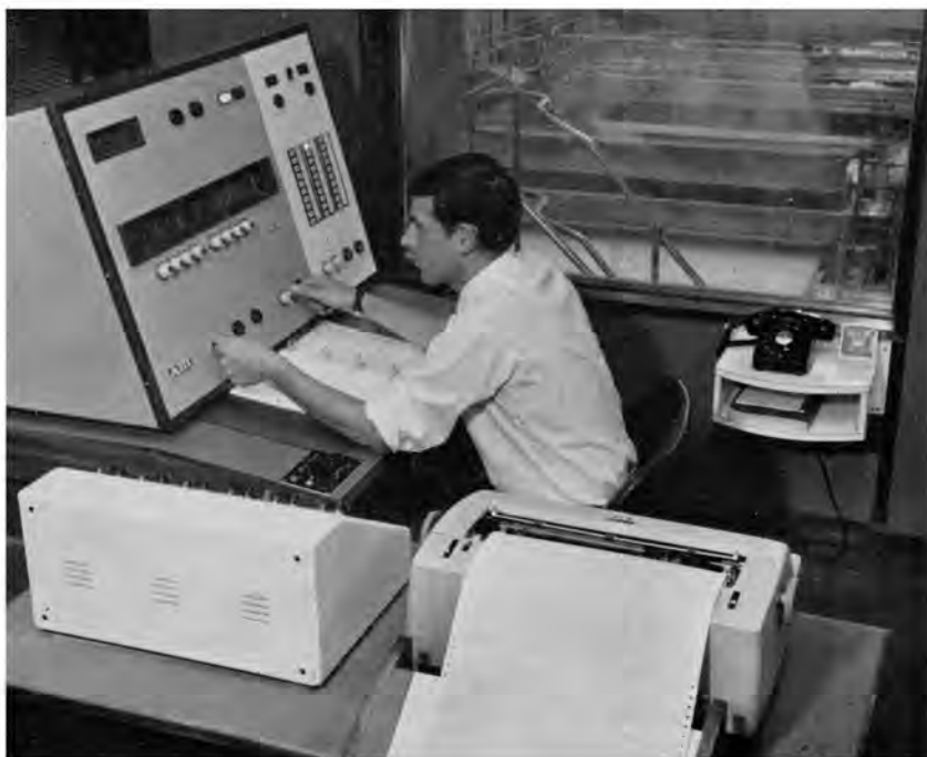
Fig. 5—Operator information and control station
